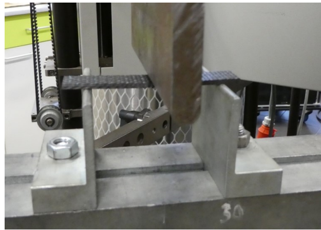
Figure 3. Three-point bending test setup.
