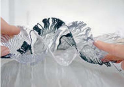
Fig. 1 Multi-layered weave: three interwoven layers of Nylon and Cotton threads result in a spatial fabric structure. Henriette Ackermann, Weißensee School of Art and Design, Berlin, Master Studio C. Sauer, 2015.
