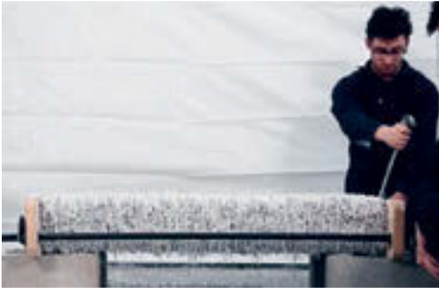
↑ The wall-slab was formed by fabricating a vertical superjammed wall, rotating into the horizontal.
