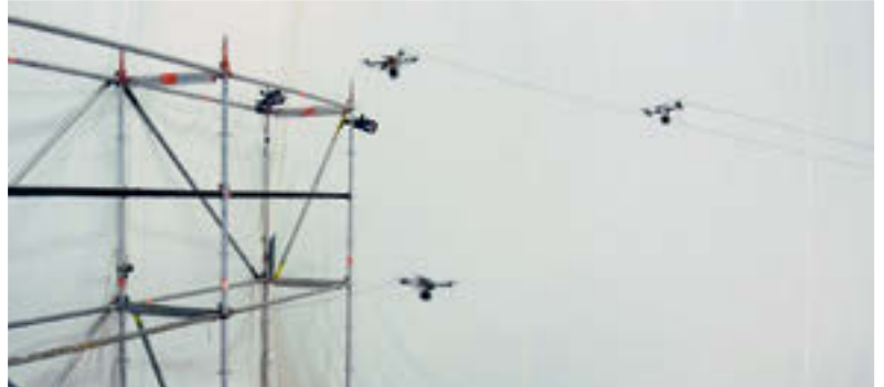
↑ Simultaneous erection of the three main links by three vehicles. Two machines start building the handrails on one side, while the third machine fixes the footrope on the other.
