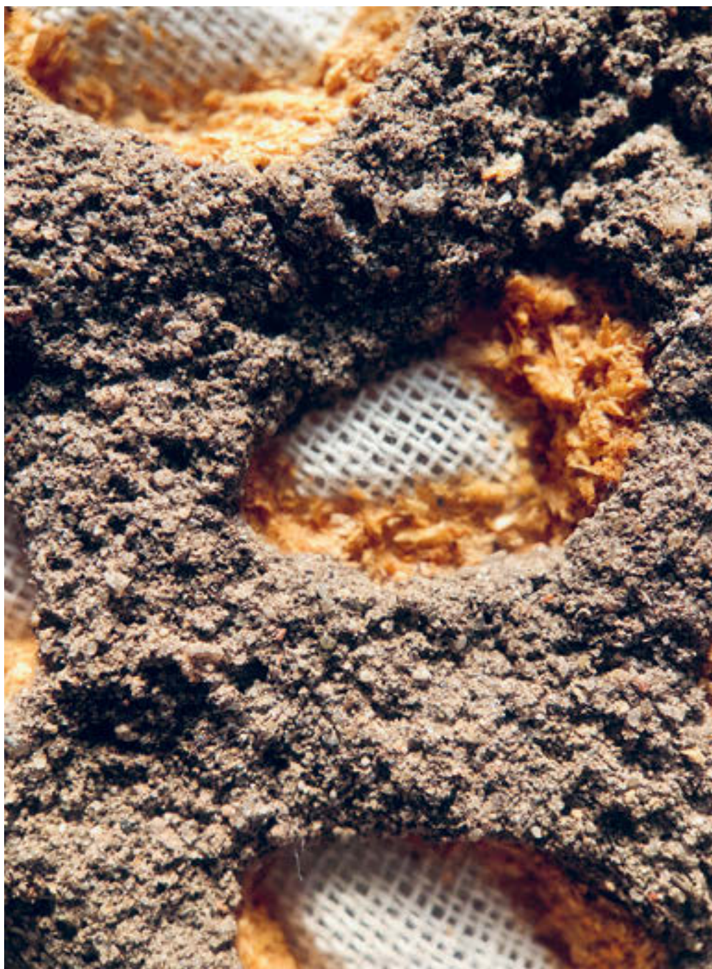
Fig. 1 A close-up of a one-sided single-layered circular pattern with two biopolymers, the dark brown based on soil, the bright brown based on sawdust.
