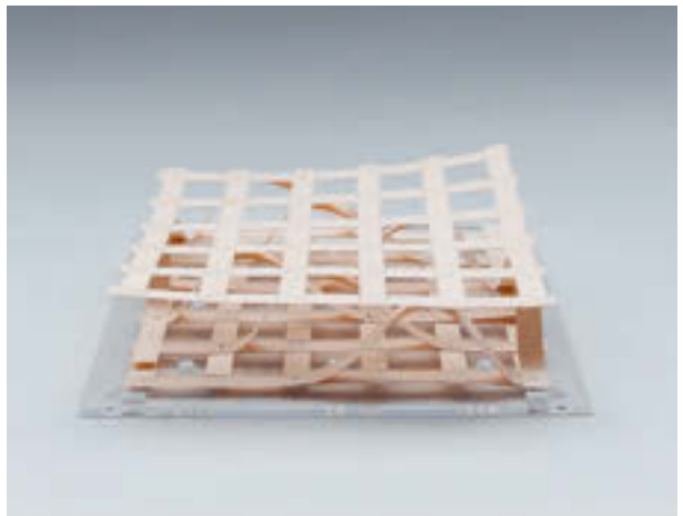
↓ 3D wood lattice made with solid maple veneer filament.
