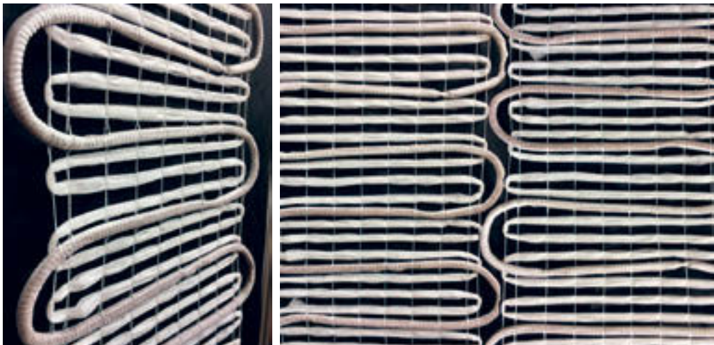
Fig. 2-3 Thermal Screens with integrated PCM yarns, processed by Kemafil ® and coarse warp-knitting technologies, creating a flexible thermal boundary.
