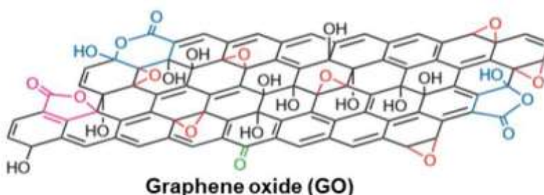
Figure 2.5, Latest structural model for graphene oxide. Only the structural connectivity is shown and steric orientations are not demonstrated. The blue colored groups demonstrate
