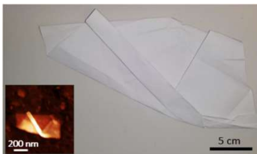
Figure 5.3, Macroscale model of a folded and wrinkled 2DTSs as seen in the inset SFM-QNM height image of the 2DTSs Nanosheet. Adapted from reference 133 .
