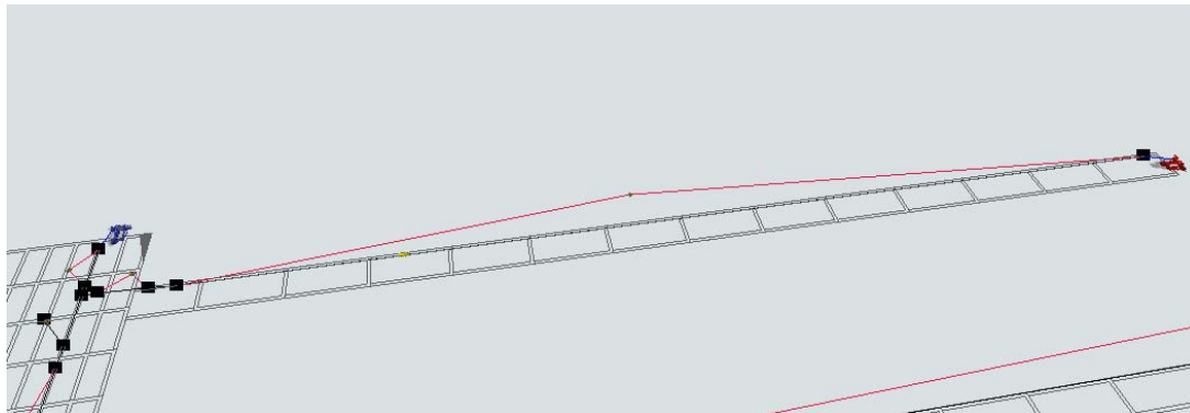
Figure 6: A single Gateroad traffic control section to allow only one large diesel delivery LHD to travel down it
