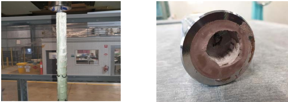
Figure 8: Failure mode of the FRP samples
