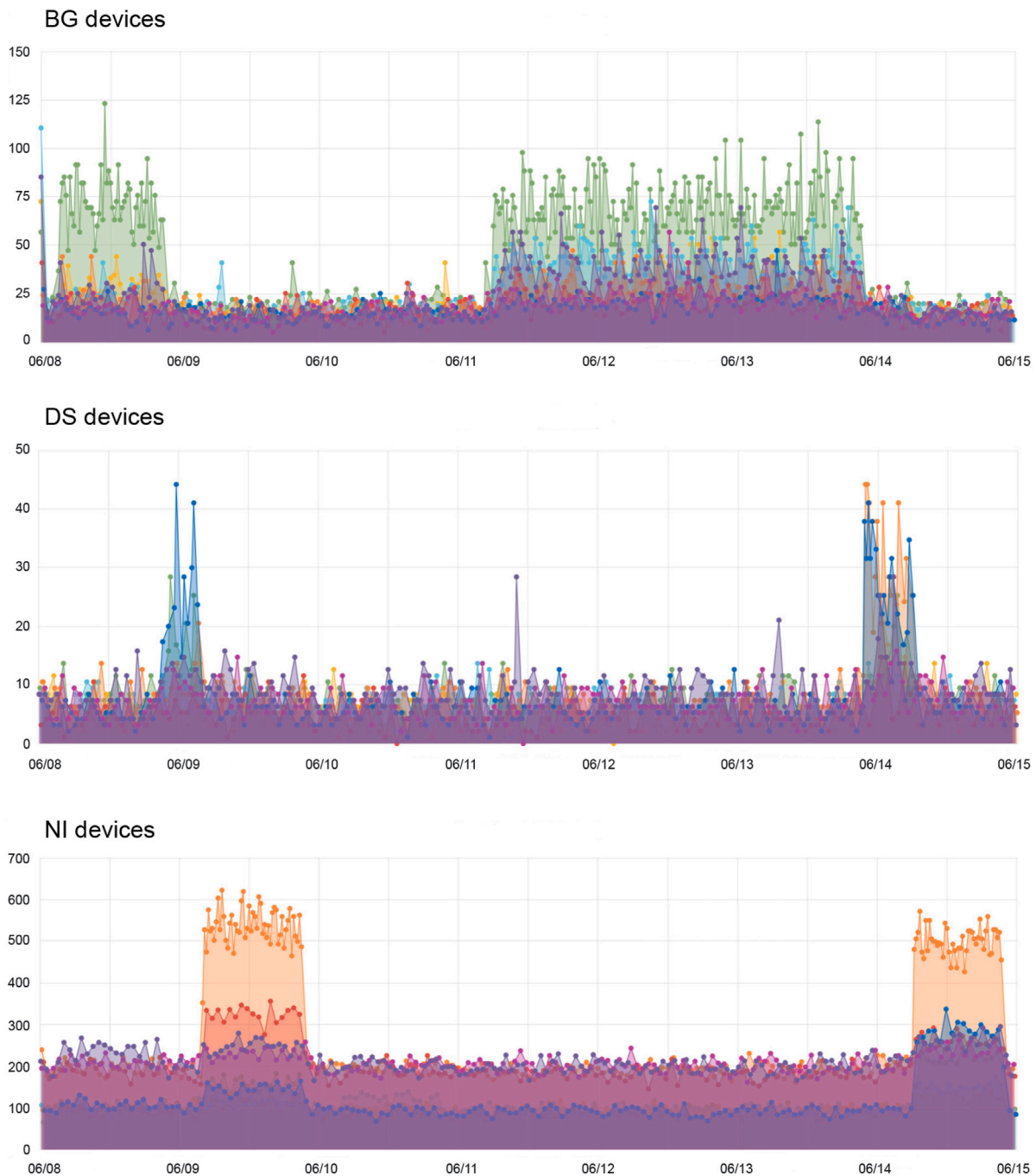
Fig. 9. Monitoring tool output showing the normalized rate for the period of the random placement tests for BG, DS and NI devices respectively. Each subfigure shows the eight devices used in different colors. We notice that some of the samples were undoubtedly detected by the W-MON system while other samples with lower activity were not able to set the alarm by surpassing the threshold. These samples were mostly samples 1 and 2. Tables 5–7 show the detailed results.
