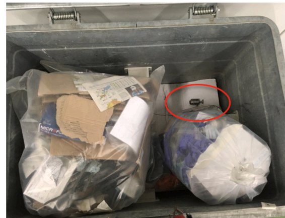
Fig. 8. Radioactive sample placed randomly in a container filled with ordinary waste.
