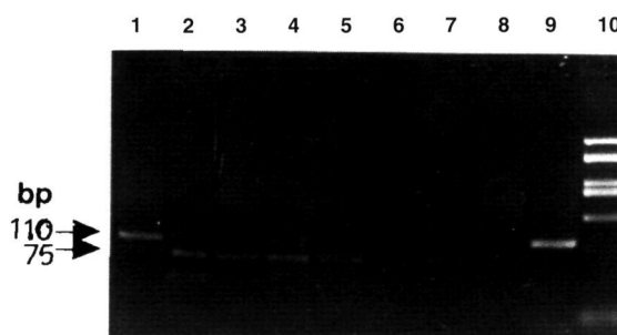
Figure 3. Detection of p53 codon 249 mutations by PCR-RFLP. PCR products after digestion with HaeIII were electrophoresed through a 2% agarose gel. Lanes 1, 9: positive controls, lanes 2, 3, 4, 5: positive samples, lanes 6, 7, 8: negative samples, lane 10: pUC18/HaeIII molecular marker.
