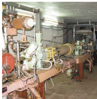
Fig. 2. Placement of SCWCL in the bunker room of the LPE-10 electron linac
