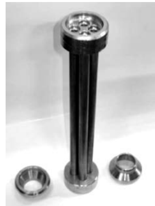
Fig. 3. Details of the 4-channel camera for SCWCL
