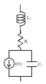
Figure 8.7: RTD model with series resistance  $R_s$ .  $C_n$  is the device capacitance and I(V) is the voltage controlled current source.
