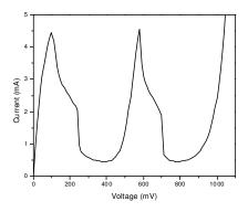
Figure 6.3: Measured I-V characteristics of two NDR devices (1N3717) connected in series. The I-V characteristic is not stretched along the voltage axis as expected due to DC instability.
