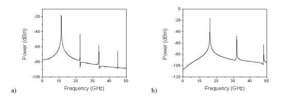
Figure 7.6: Simulated spectrum of a single RTD oscillator (400  $\mu$ m<sup>2</sup>, device size) using a fitted *I-V* characteristic: a) Fundamental oscillations are at 11.26 GHz with -18.27 dBm output power with a 500  $\mu$ m long CPW and 3.6 pF capacitor. b) Fundamental oscillations are at 16.07 GHz with -14.32 dBm output power with a 500  $\mu$ m long CPW and 2 pF capacitor.
