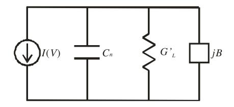
Figure 8.10: Parallel RTD oscillator with equivalent load conductance  $G'_L$  and equivalent parallel susceptance B.
