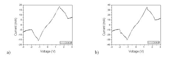
Figure 7.11: Measured RTD *I-V* characteristics with: a)  $15 \times 15 \ \mu m^2$  active area, b)  $20 \times 20 \ \mu m^2$  active area.
