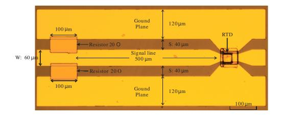
Figure 7.10: An optical picture of a fabricated MMIC RTD oscillator: a RTD with  $15 \times 15 \ \mu m^2$  active area and a DC stabiliser (two 20- $\Omega$  resistors with width = 100  $\mu$ m, length = 40  $\mu$ m and thickness = 33 nm in parallel) placed in a coplanar waveguide (CPW) line on an InP substrate with a dielectric constant of 12.56 and a thickness of 320  $\mu$ m. Signal line width, W = 60  $\mu$ m, gap space, S = 40  $\mu$ m and width of the ground planes, 120  $\mu$ m.
