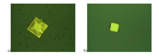
Figure 7.7: The collector after the etching process. a) a broken collector after only wet etching from the collector layer to the emitter layer, b) a good collector after both wet & dry etching from the collector to emitter layer.
