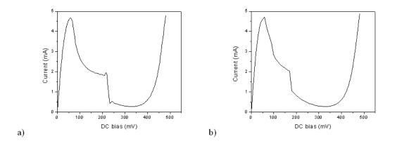
Figure 3.9: Measured current-voltage (I-V) characteristics for tunnel diodes 1N3717: a) tunnel diode 1N3717 with  $R_e = 4 \Omega$ , b) tunnel diode 1N3717 with  $R_e = 36 \Omega$ . Both I-V characteristics were modified by oscillations during the measurement.
