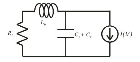
Figure 3.5: Low frequency equivalent circuit of Fig. 3.4.  $R_b$  and  $L_b$  model the resistance and inductance of the DC power supply and the bias line, respectively. I(V) and  $C_n$  model the voltage controlled current source and capacitance of the NDR device, respectively.  $C_e$  is the external capacitor in series with  $R_e$  in Fig. 3.4.
