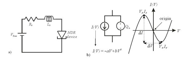
Figure 2.3: (a) A NDR device with DC bias, (b) A large-signal model for the NDR device biased in the NDR region. The voltage controlled current source I(V) is modelled by a cubic polynomial. The charge an the pn junction is modelled by a charge source  $Q_n(V)$ .
