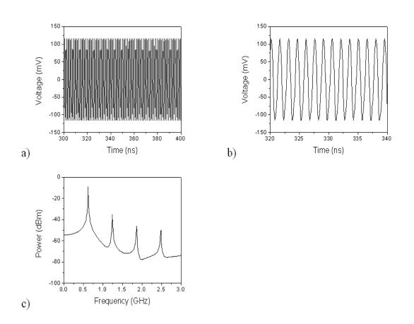
Figure 5.3: Simulation results of the tunnel diode bias circuit with the same conditions as shown in Fig. 5.2. (a) Time domain signal of the voltage across the load  $R_L$ . (b) The voltage across the load  $R_L$  between 320 ns and 340 ns. (c) The spectrum of the voltage across the  $R_L$ . The circuit oscillates at high frequency (625 MHz) determined by series inductor (L = 4 nH) and tunnel diode capacitance  $C_n$ .
