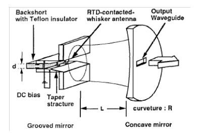
Figure 1.7: Configuration for RTD power combining in a quasi-optical resonator, after [86].
