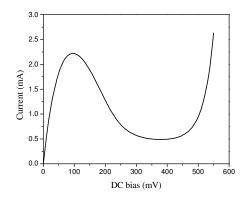
Figure 3.8: Measured current-voltage (I-V) characteristics for tunnel diode 1N3714 using the circuit in Fig. 3.4  $R_e = 20 \Omega$ ,  $C_e = 6 nF$ . The measured I-V curve seems free from oscillations.
