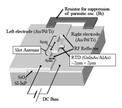
Figure 5.15: A planar resistor-stabilised millimetre-wave and THz RTD oscillator integrated with a slot antenna load [36].
