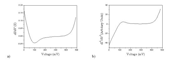
Figure 3.11: First (a) and second (b) derivatives of the *I-V* curve of the stabilised 1N3717 tunnel diode (Fig. 3.7(b)). Here  $R_e = 15 \ \Omega$ . There are no sharp valleys followed immediately by sharp peaks in the second derivative showing no oscillations are present during measurement.
