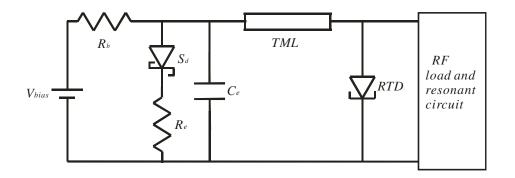
Figure 5.14: Reddy's bias stabilization scheme for sub-mm-wave RTD oscillators.  $R_b$  is the resistance of the bias line.  $S_d$ ,  $R_e$  and  $C_e$  are the Schottky diode, external resistor and external capacitor, respectively, which form the stabilising circuit. TML is the quarter-wave length transmission line at oscillation frequency [83].
