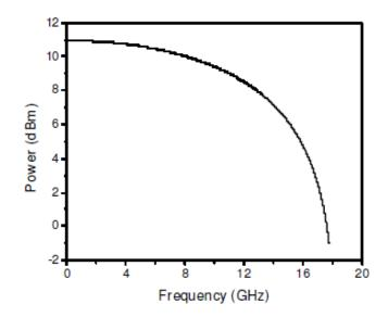
Figure 8.12: Simulated output power versus frequency for RTD layer structure used in the MMIC oscillators described in Chapter 7, Table 7.1.
