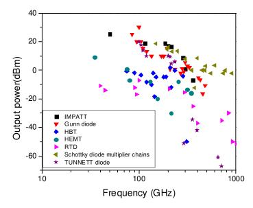
Figure 1.1: Published state-of-the-art RF power levels for IMPATT diodes, Gunn diodes, HBTs, HEMTs, RTDs, Schottky diode multiplier chains and TUNNETT diodes in the frequency range of 10 – 1000 GHz [9]-[38].
