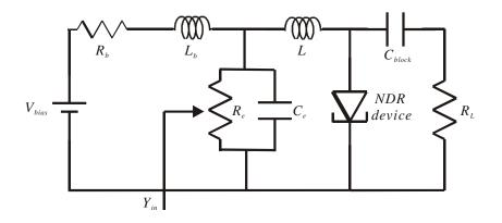
Figure 5.1: A NDR device oscillator topology with the DC decoupling circuit  $(R_e, C_e)$ .  $R_b$  and  $L_b$  model the resistance and inductance of the bias line.  $C_{block}$  and  $R_L$  are DC block and load, respectively. The total inductance L and capacitance of the NDR device determine the frequency of oscillation.
