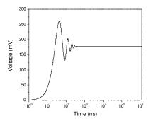
Figure 5.2: Simulation result of the tunnel diode oscillator with  $R_e < 1/G_n$ .  $R_b = 1 \Omega$ ,  $L_b = 56 \text{ nH}, L = 4 \text{ nH}, R_e = 15 \Omega, C_e = 2.5 \text{ nF}, R_L = 50 \Omega, C_{block} = 2.5 \text{ nF}$  and  $V_{bias}$  = 180 mV. It shows the time domain signal of the voltage across the shunt resistor  $R_e$ . The voltage across  $R_e$ , which is the same as across the bias line, is constant with time indicating that no bias oscillations are present.
