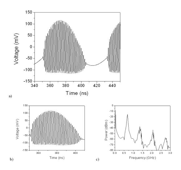
Figure 5.5: Simulation results of the tunnel diode bias circuit with the same conditions as shown in Fig. 5.4. (a) Time domain signal of the voltage across the load  $R_L$ . (b) Time domain signal of the voltage across the load  $R_L$  between 350 ns and 410 ns. (c) The spectrum of the voltage across  $R_L$ .
