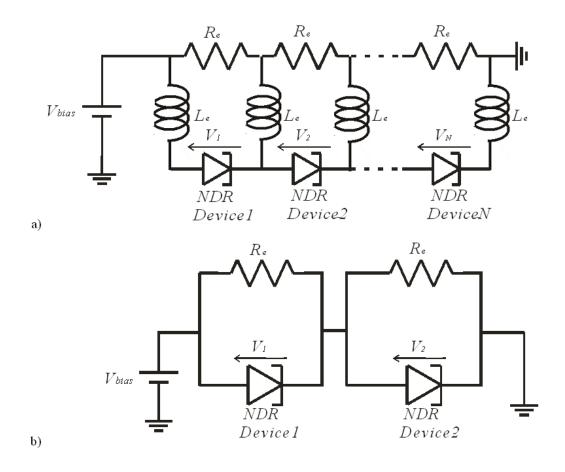
Figure 6.6: a) Circuit diagram of the series integration of N NDR devices and external stabilizing resistors  $(R_e)$  that are connected to the NDR devices through external inductors  $(L_e)$ , b) Two series-connected NDR devices with external stabilising resistors  $(R_e)$ .
