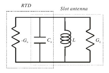
Figure 5.16: RF equivalent circuit of Figure 5.15 [36].
