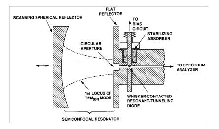
Figure 1.5: Schematic cross-sectional diagram of a quasioptical waveguide resonant tunnelling diode oscillator, after [40].
