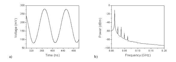
Figure 5.4: Simulation results of the tunnel diode oscillator with  $R_e > 1/G_n$ .  $R_b = 1$  $\Omega$ ,  $L_b = 56$  nH, L = 0 nH,  $R_e = 50 \Omega$ ,  $C_e = 2.5$  nF,  $R_L = 50 \Omega$ ,  $C_{block} = 2.5$  nF and  $V_{bias} = 180$  mV. (a) Time domain signal of the voltage across the shunt resistor  $R_e$ . (b) The spectrum of the voltage across  $R_e$ .
