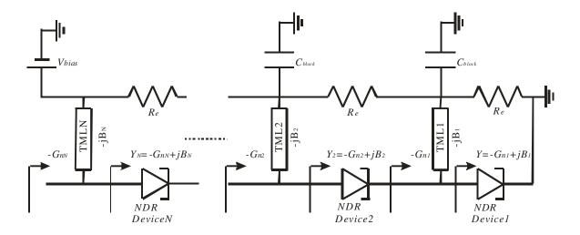
Figure 6.10: An extended resonance power combining circuit topology with N NDR devices connected in series. TML are transmission lines.
