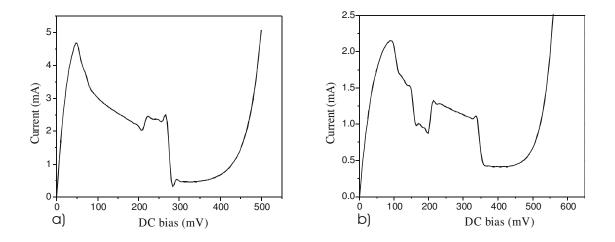
Figure 3.6: Measured I-V characteristics for a) tunnel diode 1N3717 and b) tunnel diode 1N3714 without bias and high frequency stabilisation. The curves in the NDR region have the characteristic 'plateau' distortion due to bias oscillations.
