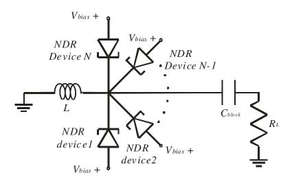
Figure 9.1: A N tunnel diodes/RTDs parallel-connected oscillator topology with individual DC decoupling circuit for each device.
