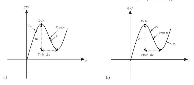
Figure 6.7: Possible bias points for two series-connected NDR devices having a bias supply capable of biasing both in the mid-points of the NDR regions. a)  $V_1 > V_{NDR}M$ b)  $V_1 < V_{NDR}M$ .
