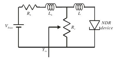
Figure 2.5: A NDR device oscillator topology with the DC decoupling circuit  $(R_e)$ .  $R_b$ and  $L_b$  model the resistance and inductance of the DC power supply and the bias line, respectively. The inductance L and self-capacitance of the NDR device can lead to high frequency oscillations in the circuit.
