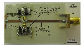
Figure 5.9: A picture of a two tunnel diodes (1N3717) parallel-connected oscillator realized in hybrid microstrip technology.
