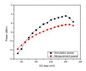
Figure 5.12: The measured and simulated output power of the two tunnel diode parallelconnected oscillator as a function of bias voltage.
