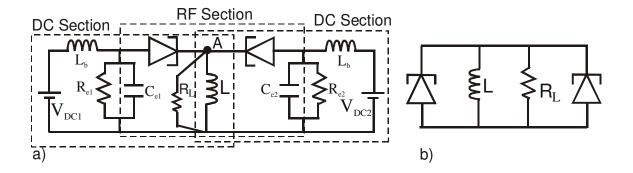
Figure 5.7: a) A two tunnel diode parallel-connected oscillator topology with DC stabilisers  $C_{e1}$ ,  $R_{e1}$ ,  $C_{e2}$  and  $R_{e2}$  ( $R_{e1} < 1/G_n$  and  $R_{e2} < 1/G_n$ ), the inductance L, DC block  $C_{block}$  and 50  $\Omega$  load  $R_L$ . In both circuits the output power is taken from node A thereby establishing a parallel resonant circuit. b) RF equivelent circuit.
