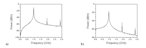
Figure 8.5: Simulation results of the tunnel diode oscillator with  $R_e < 1/G_n$ .  $R_b = 1 \Omega$ ,  $L_b = 56 \text{ nH}, L = 2 \text{ nH}, R_e = 10 \Omega, C_e = 2.5 \text{ nF}, R_L = 50 \Omega, C_{block} = 2.5 \text{ nF}$  and  $V_{bias}$  = 180 mV. a) The power delivered to the load  $(R_L)$  at 935 MHz is -10.8 dBm with an RF short circuit via  $C_e = 2.5 \text{ nF}$ . b) The power delivered to the load  $(R_L)$  at 935 MHz is -17.6 dBm without  $C_e$ .
