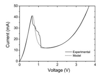
Figure 7.5: Experimental and modelled *I-V* characteristics for the RTD (400  $\mu$ m<sup>2</sup>) with capacitance  $C_n = 3.6$  pF [103].
