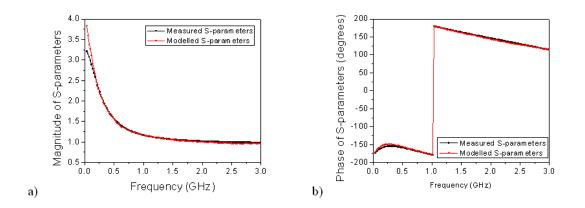
Figure 4.6: The measured (converted from measured Y-parameters,  $Y_{12}$  or  $Y_{21}$ ) and modeled s-parameters of the tunnel diode in the NDR region at 140 mV, a) Comparison between measured and modelled magnitude of the s-parameters, b) Comparison between measured and modelled phase of the s-parameters.
