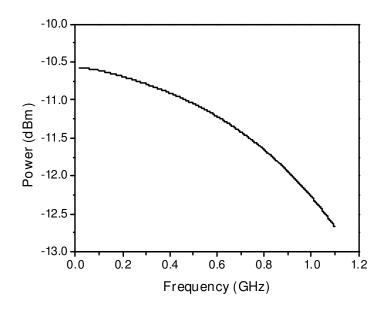
Figure 8.11: Simulated output power versus frequency for the 1N3717 tunnel diode.
