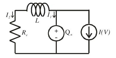
Figure 2.6: Large-signal RF equivalent circuit of Fig. 2.5. The bias line inductance  $L_b$  in Fig. 2.5 is assumed large and so decouples the RF signal from the DC supply.
