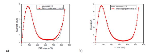
Figure 6.5: a) Measured I-V characteristic (continuous trace) of the tunnel diode (1N3717) and an eighth-order polynomial fit (dotted trace). b) Measured I-V characteristic of the tunnel diode (1N3717) and a ninth-order polynomial fit.
