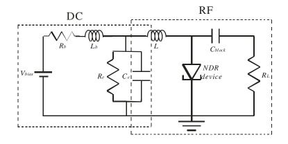
Figure 8.3: RTD oscillator with RF and DC separated by DC decoupling circuit ( $R_e$ ,  $C_e$ ).  $R_L$  is the load of the RTD oscillator. The inductance L and self-capacitance of the NDR device determine the frequency of oscillation.
