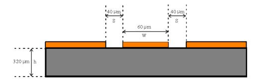
Figure 7.2: Cross-section of a CPW on an InP substrate with a dielectric constant of 12.56 and a thickness of 320  $\mu$ m. The signal line width W = 60  $\mu$ m, and the gap space S = 40  $\mu$ m.
