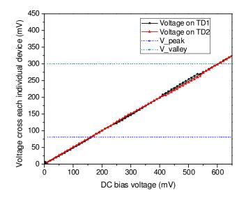
Figure 6.8: Measured voltages across two individual tunnel diodes (1N3717) in the series integration as shown in Fig. 6.6(b). The measurements show that the bias voltage is almost evenly split between the two devices.
