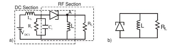
Figure 5.6: a) A single NDR device oscillator topology with DC stabilisers  $C_e$  and  $R_e$  $(R_e < 1/G_n)$ , oscillation frequency determining inductance L, and load resistance  $R_L$ . b) RF equivalent circuit
