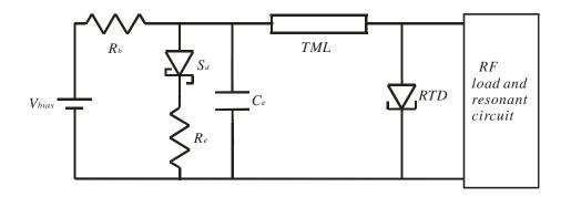
Figure 1.6: Reddy's bias stabilization scheme for sub-mm-wave RTD oscillators.  $R_b$  is the resistance of the bias line.  $S_d$ ,  $R_e$  and  $C_e$  are the Schottky diode, external resistor and external capacitor, respectively, which form the stabilising circuit. TML is the quarter-wave length transmission line at the oscillation frequency [83].
