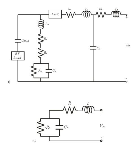
Figure 8.6: a) The equivalent circuit for a resonant tunnelling diode waveguide oscillator including the bias circuit. b) The equivalent circuit where series elements have been combined without an external capacitor [63].
