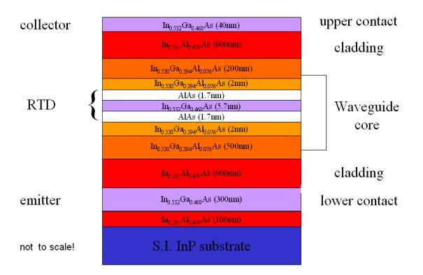
Figure 7.1: The heterolayer structure specification for the RTD-OW wafer. It was grown by Molecular Beam Expitaxy in a Varian Gen II system on a semi-insulating InP substrate by IQE, Ltd.
