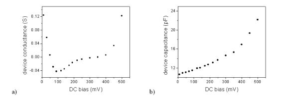
Figure 4.7: Extracted device conductance and capacitance of a tunnel diode (1N3717) with different DC bias voltages: a) The extracted device conductance, b) the extracted device capacitance.
