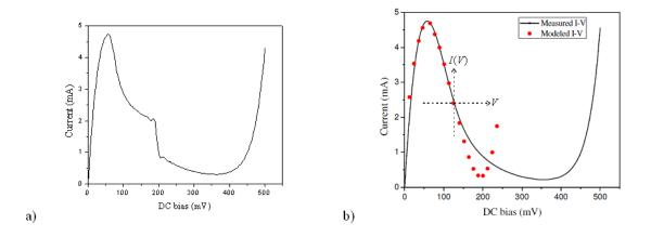
Figure 3.7: Measured current-voltage (I-V) characteristics for tunnel diodes 1N3717 using the circuit in Fig. 3.4: a) tunnel diode 1N3717 with  $R_e = 8 \ \Omega$ ,  $C_e = 6 \ nF$ , b) tunnel diode 1N3717 with  $R_e = 15 \ \Omega$ ,  $C_e = 6 \ nF$ . (a) contains oscillations while (b) is free from oscillations. The measured I-V curve in (b) has also been fitted with the cubic polynomial, showing a good fit (dots) to measured data (solid line) in the NDR region (except the broad valley region).
