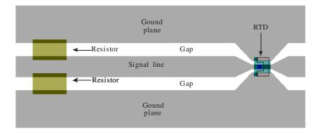
Figure 7.4: Layout of MMIC RTD oscillator comprising an RTD and a DC decoupling circuit (two resistors in parallel) embedded in a coplanar waveguide (CPW) line. The characteristic impedance of the CPW is 50  $\Omega$  and its series inductance per unit length is 90 pH/mm. The output power can be measured from the right hand side using a 50- $\Omega$  CPW probe.
