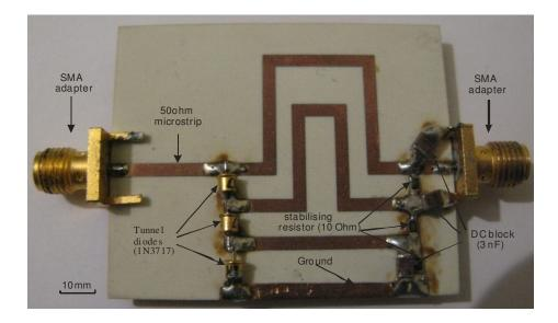
Figure 6.12: A picture of the three series-connected tunnel diodes (1N3717) oscillator realised in hybrid microstrip technology.
