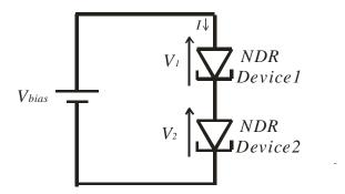
Figure 6.1: A diagram of two NDR devices connected in series
