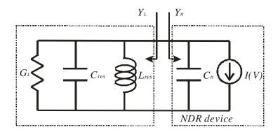
Figure 8.1: A large-signal RF equivalent circuit of parallel RTD oscillator with load conductance  $G_L$  and resonant circuit (inductance  $L_{res}$  and capacitance  $C_{res}$ ).
