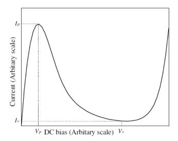
Figure 1.3: Typical current-voltage characteristic of a tunnel diode [46].
