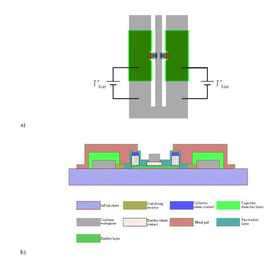
Figure 9.2: Top view (a) and the cross-section (b) of an illustration of a MMIC oscillator employing two RTDs.
