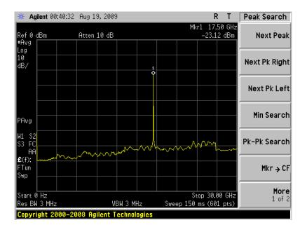
Figure 7.12: Picture of measured spectrum of the fabricated oscillator with  $15 \times 15 \ \mu m^2$ RTD active area and 500  $\mu m$  long CPW lines. Spectrum shows fundamental oscillation frequency is 17.5 GHz and output power is of -23.12 dBm.
