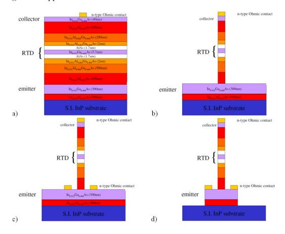
Figure 7.8: Cross-sectional views of the main fabrication steps for the RTD.
