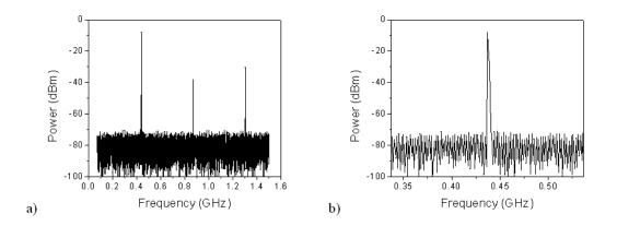
Figure 5.11: a) The measured spectrum of a two tunnel diode parallel-connected oscillator with -7.83 dBm fundamental oscillations at 437 MHz. b) An expanded spectrum of Fig. 5.11(a) around the fundamental oscillations frequency.
