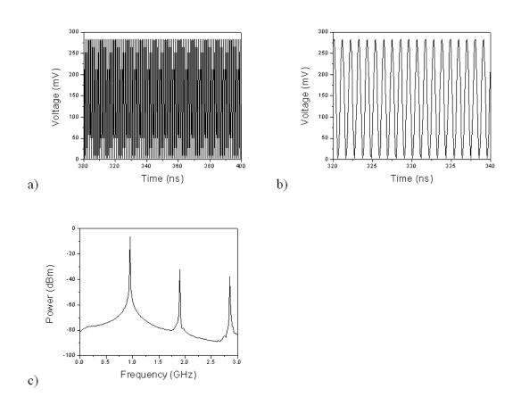
Figure 3.2: Simulation results of the tunnel diode bias circuit with  $R_e < 1/G_n$ .  $R_b = 1 \ \Omega$ ,  $L_b = 56 \ \text{nH}$ ,  $L = 2 \ \text{nH}$ ,  $R_e = 5 \ \Omega$  and  $V_{bias} = 170 \ \text{mV}$  (the DC voltage across the tunnel diode is 140 mV). (a) Time domain signals of the voltage across the load  $R_L$  over a 100 ns time span, (b) Time domain signals of the voltage across the load  $R_L$  over a 25 ns time span, (c) The spectrum of the diode voltage.
