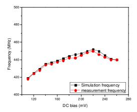
Figure 5.13: The measured and simulated oscillation frequencies of the two tunnel diode parallel-connected oscillator as a function of bias voltage.
