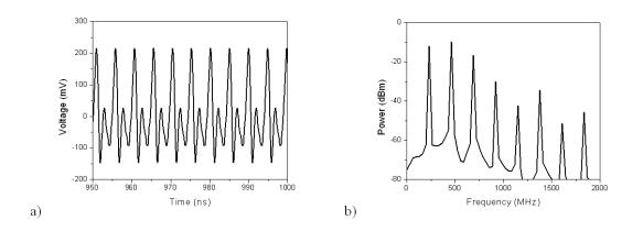
Figure 6.15: Transient/time domain simulation results for oscillator with three tunnel diodes connected in series using the extended resonance technique. (a) Time domain signal of the voltage across the 50- $\Omega$  load. (b) The spectrum of the voltage across the 50  $\Omega$  load obtained using a in-built "fs" function in ADS.
