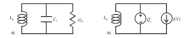
Figure 2.4: (a) A small-signal equivalent circuit of Fig.2.3(a).  $R_b$ ,  $R_s$  and  $L_s$  are typically small therefore they are ignored in the RF equivalent circuit, (b) A large-signal RF equivalent circuit of Fig. 2.3(a).
