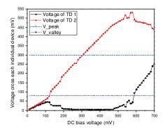
Figure 6.4: Measured voltages across two individual tunnel diodes (1N3717) in the series integration as shown in Fig. 6.1. The voltage range between two dashed lines  $V\_peak$ and  $V\_valley$  is the NDR region for a single device. It shows that the bias voltage is not evenly split between the two devices but is divided such that either one or both of the devices are in the positive differential resistance (PDR) region.
