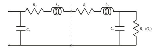
Figure 4.5: Small-signal equivalent circuit of an NDR device (including the package parasitic) with  $L_s + L_p = 1.61$  nH,  $R_p + R_s = 1.09 \Omega$ ,  $C_p = 0.41$  pF,  $C_n = 12.42$  pF and  $-G_n = -0.035 S$  when it was biased at 140 mV.
