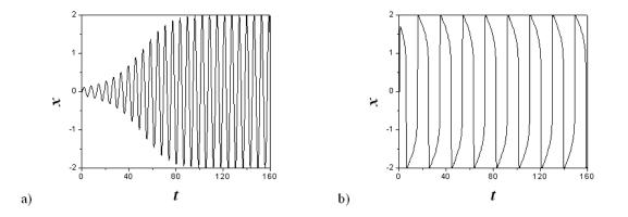
Figure 2.1: Solutions to the Van der Pol equation (2.1) for positive values of  $\varepsilon$ . (a) Oscillation waveform with  $\varepsilon = 0.1$ , (b) Oscillation waveform with  $\varepsilon = 10$ .
