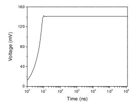
Figure 3.3: Time domain simulation results of the tunnel diode bias circuit with  $aL/C_n$  $< R_e < 1/a$ .  $R_b = 1 \Omega$ ,  $L_b = 56 \text{ nH}$ , L = 2 nH,  $R_e = 15 \Omega$ , and  $V_{bias} = 155 \text{ mV}$  (the DC voltage across the tunnel diode is 140 mV). It shows that neither low-frequency bias oscillations nor high frequency oscillations are present.
