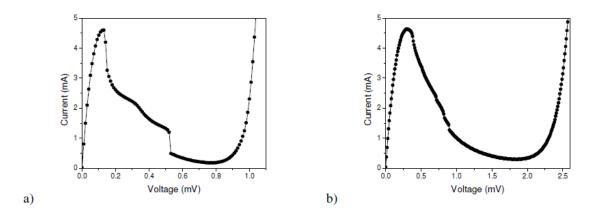
Figure 6.9: Extracted I-V characteristics of a) 2 and b) 5 tunnel diodes (1N3717) connected in series. Compared to the I-V characteristics of a single device as shown in Fig. 3.7(b), the voltage axis is expanded 2 and 5 times, respectively.
