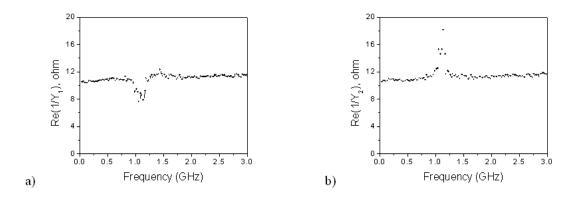
Figure 4.3: Real part of the stabilising resistive elements  $R_1$  and  $R_2$ . The peak and trough in the measurement are assumed to be due to resonance caused by the inductance of the microstrip lines and the diode package capacitance.
