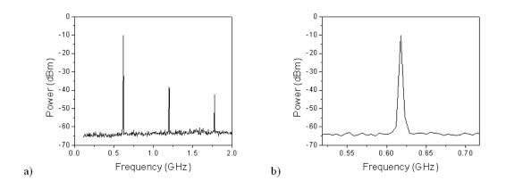
Figure 5.10: a) The measured spectrum of a single tunnel diode oscillator with fundamental oscillations at 618 MHz with -10.17 dBm output power. b)An expanded spectrum of Fig. 5.10(a) around the fundamental oscillations frequency.
