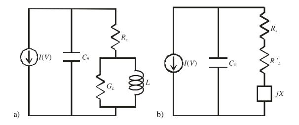
Figure 8.9: Re-drawn RF equivalent circuit of the circuit of Fig.8.8.
