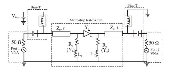
Figure 4.2: Schematic of the measurement set-up for s-parameter characterisation of an NDR device. Resistors  $R_1$  and  $R_2$  are chosen to cancel the negative conductance of the NDR device and so ensure circuit stability during characterisation.
