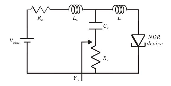
Figure 3.4: A circuit for direct *I-V* measurement of tunnel diodes or general NDR devices. An external capacitor  $C_e$  is introduced in series with  $R_e$ . Circuit stability is determined by equation (3.1). Transient simulations showed stability with  $C_e = 6$  nF.
