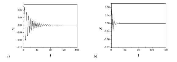
Figure 2.2: Solutions to the Van der Pol equation (2.1) for negative values of  $\varepsilon$ . (a) Oscillation waveform with  $\varepsilon = -0.1$ , (b) Oscillation waveform with  $\varepsilon = -0.5$ .
