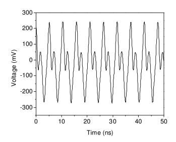
Figure 6.13: Measured waveform of the three series-connected tunnel diodes (1N3717) oscillator.
