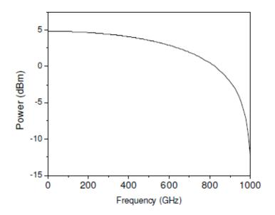
Figure 8.13: Simulated output power versus frequency for RTD layer structure in Ref. [36].
