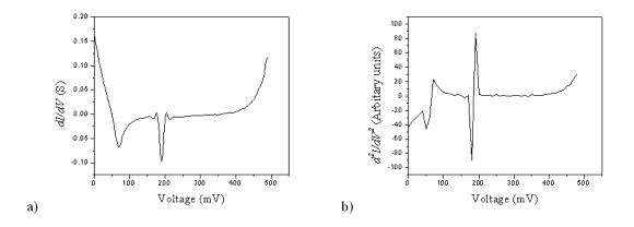
Figure 3.10: First (a) and second (b) derivatives of the *I-V* curve of the 'stabilised' 1N3717 tunnel diode (Fig. 3.7(a)). Here  $R_e = 8 \Omega$ . The valley/peak in the second derivative shows the presence of oscillations in the 90 mV to 180 mV range of the NDR region.
