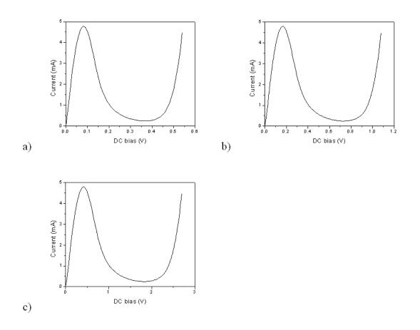
Figure 6.2: a) Measured I-V characteristic of single NDR device (1N3717), b) Simulated ideal I-V characteristic of 2 NDR devices (1N3717) connected in series, c) Simulated ideal I-V characteristic of 5 NDR devices (1N3717) connected in series. Note that in b) and c), the voltage is expanded by 2 and 5 times, respectively, compared to the single device.
