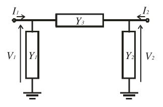
Figure 4.1: A diagram for a typical pi-network.
