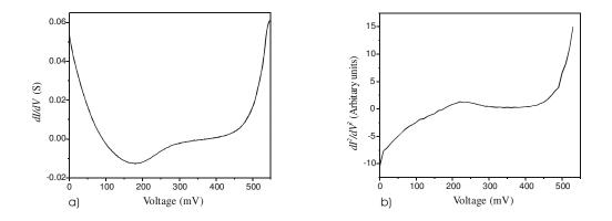
Figure 3.12: First (a) and second (b) derivatives of the I-V curve of the stabilised 1N3714 tunnel diode (Fig. 2.14(c)). There are no valleys/peaks in the second derivative showing no oscillations present during measurement.
