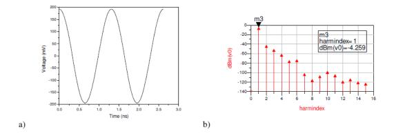
Figure 6.11: Harmonic Balance simulation results for an oscillator with 3 tunnel diodes connected in series using the extended resonance technique. (a) Time domain signal of the voltage across the 50- $\Omega$  load. (b) The spectrum of the voltage obtained using a in-built function "fs" in ADS shows an output power of -4.259 dBm at the fundamental frequency.
