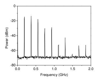
Figure 6.14: Measured spectrum of the three series-connected tunnel diodes (1N3717) oscillator.
