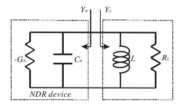
Figure 8.4: A small-signal RF equivalent circuit of Fig.8.3. The circuit can deliver maximum power to the load  $(G_L)$  if the conductance of the load is equal to half conductance of the NDR device at the bias point.
