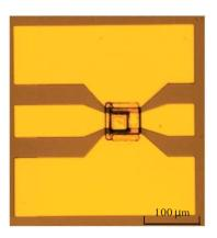
Figure 7.9: A fabricated RTD with 15×15  $\mu$ m<sup>2</sup> active area and 100  $\mu$ m CPW metal pads.
