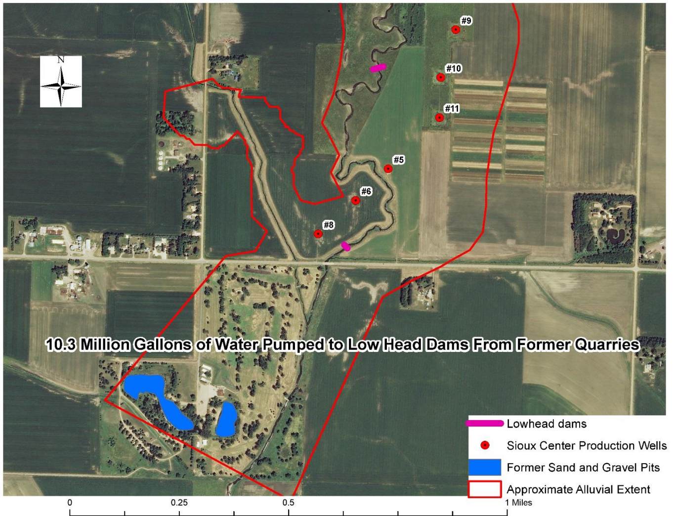
Figure 7. Former sand and gravel quarries that may be used for drought contingencies.
