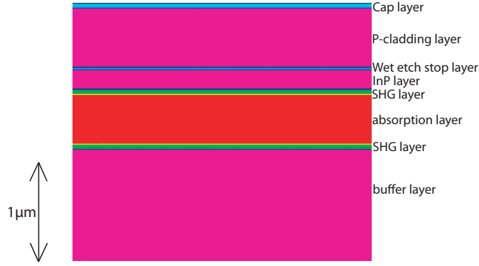
FIGURE 4.2: Composition of the wafer structure used for the TPA detectors fabrication
