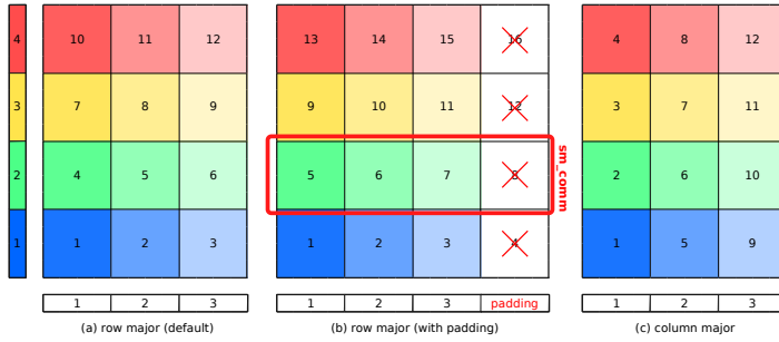
FIG. 8. Different virtual topologies to increase data locality (a) for the basis change S and (c) for the inner preconditioner. Version (b) introduces padding to guarantee that all stages are on the same shared-memory domain/same compute node.
