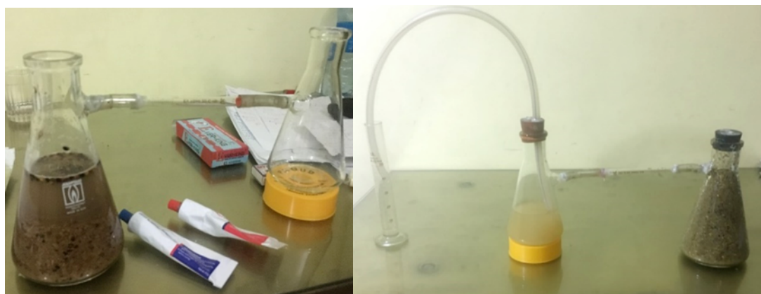
Figure 2. Water displacement setup: Slurry in flask, water in 400ml flask and measuring cylinder.
