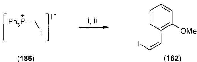
Scheme 3.3.2. Reagents and conditions: i, KHMDS, THF, rt; then ii, HMPA, o -anisaldehyde, -78°C to rt, 73%.
