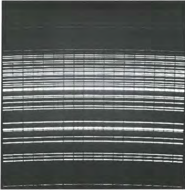
Figure 4.1: TEIFU arc lamp observation, showing the raw data format, from the September 1999 commissioning run. The 18 blocks of 56 fibre spectra are separated by gaps of \sim 3 pixels.
