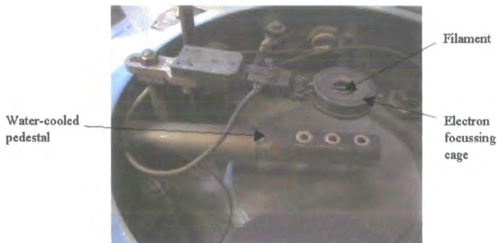
Fig. 3.4 Electron-beam source assembly
