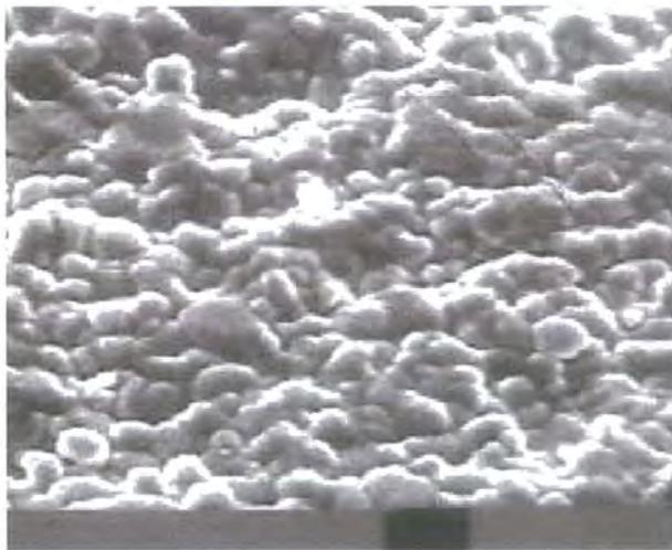
Fig. 3.21 E-beam evaporated film on Al<sub>2</sub>O<sub>3</sub>, annealed at 500°C
