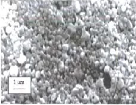
Fig. 4.13 SEM image for a film with glass phase, fired at  $850^{\circ}\text{C}$  for 30 min
