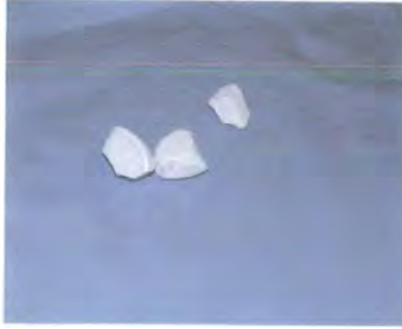
Figure 3.12 Photograph of the aluminium PolyHIPE composite.
