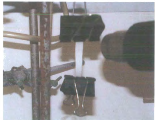
Figure 9.9 Photographs of the shape memory effect of 258RJC.
