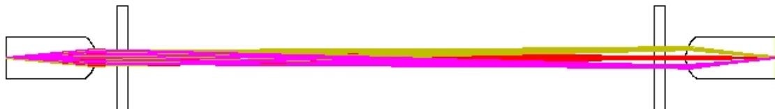
Figure 3.12: A ZEMAX ray-tracing diagram of the SALT HRS double scrambler, with identical spherical rod lenses L1 and L2 on the left and right respectively, separated by 112mm to accommodate an optional iodine cell (2mm cell windows shown 100mm apart) or fold mirror for a simultaneous Thorium-Argon source feed.
