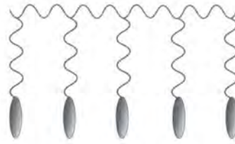
Figure 2.4: Side chain liquid crystal polymer with mesogens terminally attached to flexible spacers.
