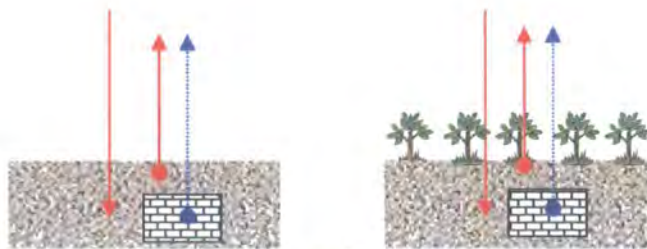
Figure 3.3: Effect of short vegetation on thermal response at the surface
