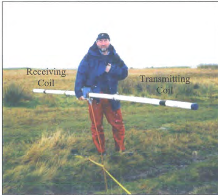
Figure 3.14: Dual-loop EM31 electromagnetic system with transmitting and receiving coils mounted on horizontal pole
