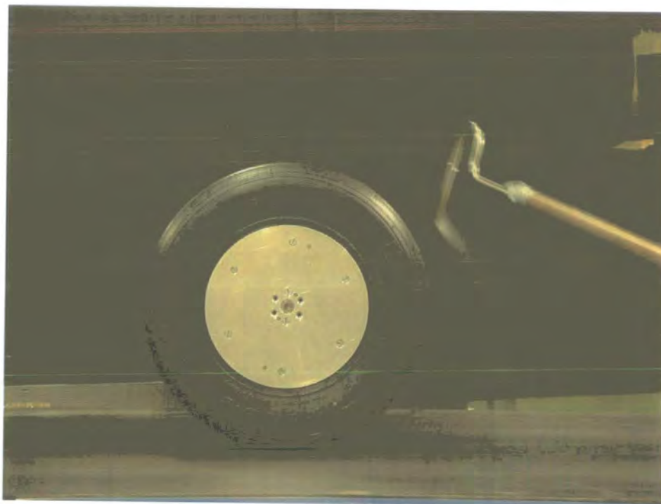
Figure 8.37: Smoke Flow Visualisation for the Stationary Wheel with the Smoke Probe Positioned on the Centreline at 225 degrees.
