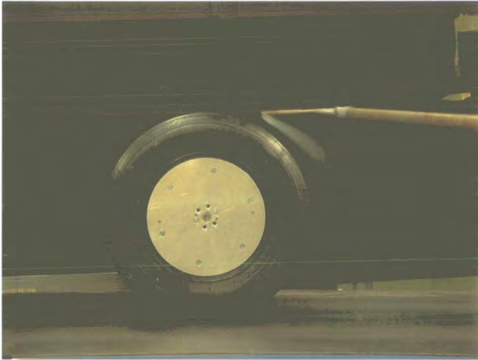
Figure 8.39: Smoke Flow Visualisation for the Stationary Wheel with the Smoke Probe Positioned on the Centreline at 250 degrees.
