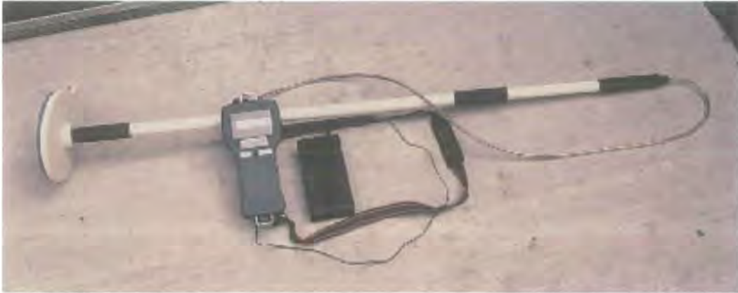
Figure 3.1 Prototype 12-mm Passive Integrated Transponder (PIT) tag reader (UKID Systems, Preston, UK), shown with external battery pack (black casing). Pole with search head measures 1.5 m.
