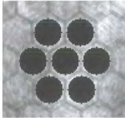
Figure 5.6: The CCD pixels are re binned to correspond to the detector pixels. The hexagonal pixels of the Hex 127 can be seen, with the black circles representing the binned detector pixels
