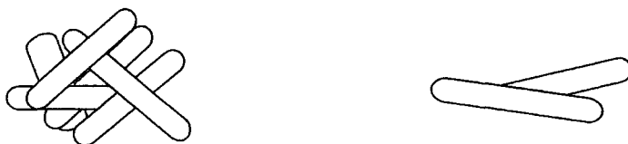
Figure 4-24. Large cluster with small or no anisotropy (left); small cluster with high anisotropy (right)
