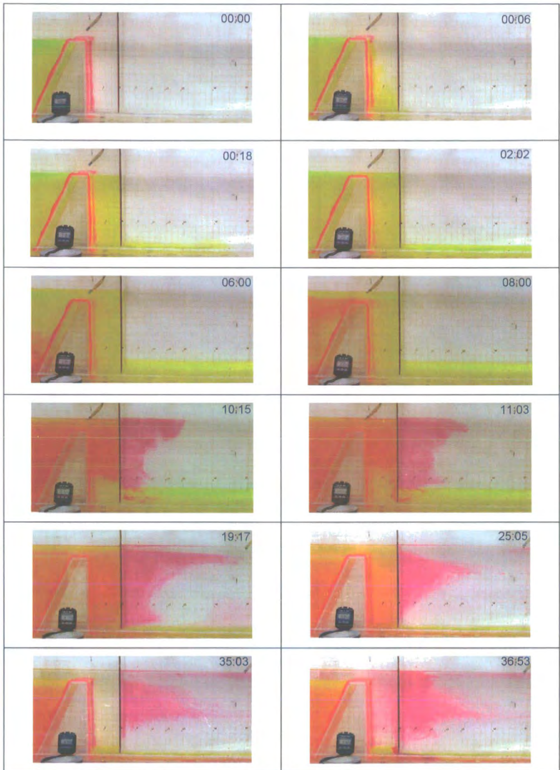
Figure 3-10 Flume experiment No. 1: Baffle, yellow dye indicates salt-water, red dye is injected to visualize hydrodynamic patterns within layers and at interfaces, first injection point is downstream of barrage in the lower layer (06:00 min.), second injection point is upstream of the baffle throughout the water column (10:15 min.)
