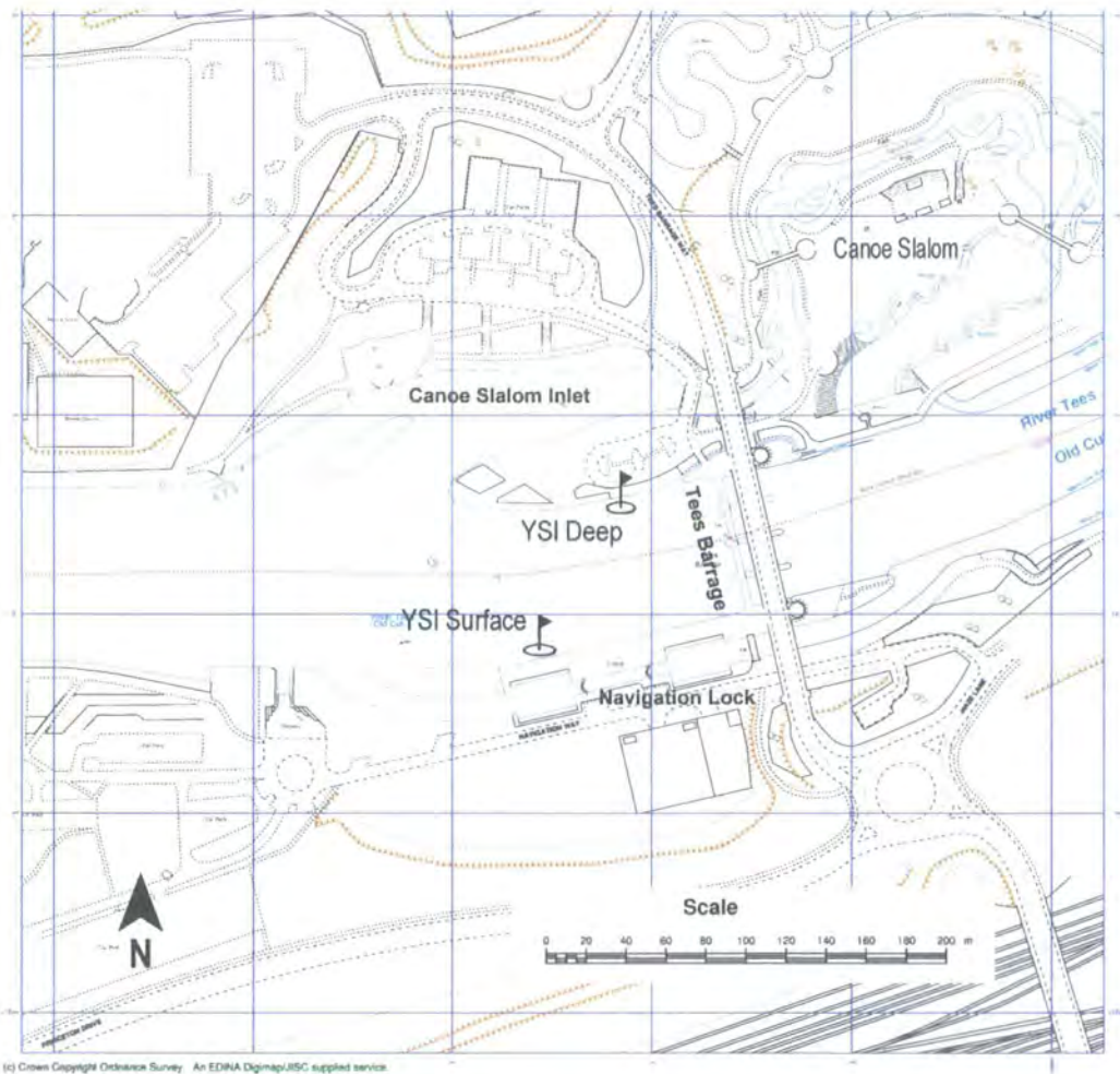
Figure 5-3 Water quality sonde locations in the Tees impoundment
