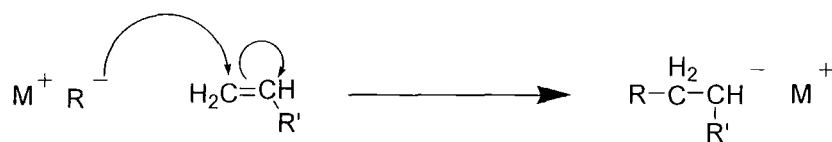
Figure 17 Anionic addition polymerisation
