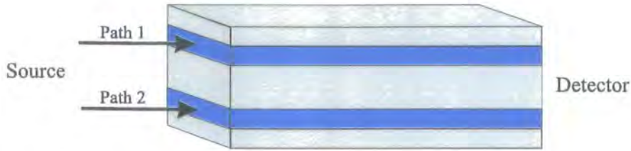
Figure 1.1: Schematic of a slab waveguide interferometer. High refractive index (turquoise) and low refractive index (grey) regions are combined to create two different optical paths. The arrangement may be used as an interferometer to allow differences between the two optical paths to be investigated.
