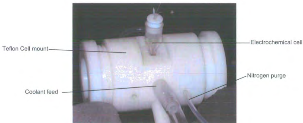
Figure 2.5. Spectro-electrochemical apparatus for UV-vis-NIR measurements
