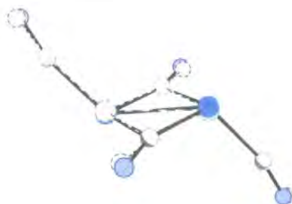
Figure 8.10: Overlay of the copper dimer at 180 K and 90 K. The high spin, 180 K structure is shown with dotted open circles and bonds drawn with a broken line. A subtle change in the orientation of the [\text{Cu}(\text{CN})_2]^- groups can clearly be seen.
