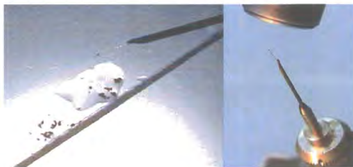
Figure 2.3: Mounting crystals using the 'oil drop' method. 132
