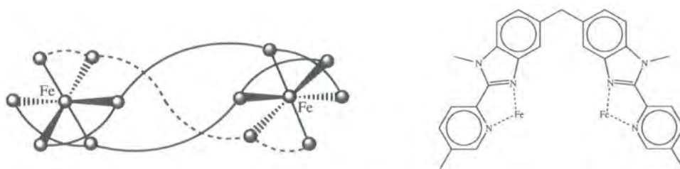
Figure 1.27: A binuclear spin crossover iron(II) helicate. A schematic of the structure is shown (left) together with the ligand (right). The ligand is tetradentate, binding twice to both iron centres (shown with broken lines). Three ligands, each binding in a bidentate arrangement round the two iron centres, combine to make the helical complex.
