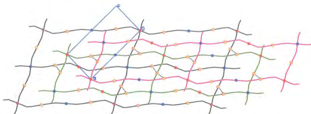
Figure 7.12: Three interpenetrating networks in compound 6 , shown in black, green and pink, viewed down the b -axis. Fe1 atoms are shown in red, Fe2 atoms are shown in blue, the aurophilic bonds are shown with broken black lines and the unit cell outline is shown in blue.
