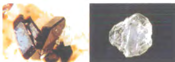
Figure 2.2: Good quality crystals and poor quality crystals. The sample on the left consists of well shaped crystals free from intergrowths and inclusions. The sample on the right has no clear faces and may contain a number of crystalline components. 129
