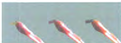
Figure 6.9: A crystal of compound 5 . At 400 K (left) the crystal is clear pale yellow, but on cooling to 250 K the colour darkens to a deep orange (centre) and cooling to 100 K gives a dark red colour (right).
