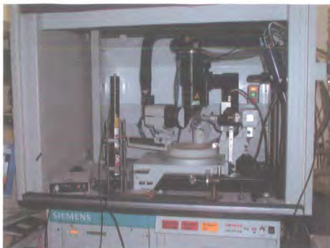
Figure 1.3-1 The SMART 1000 as found in the Durham crystallography laboratory. In this diagram, the Oxford Cryosystems' 'HeliX' is being used.
