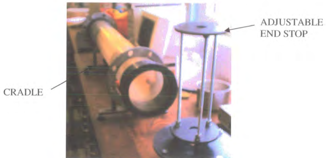
Figure 5.51. Casting apparatus for annular bypass wax removal tests.
