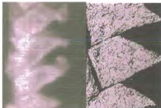
Figure 4.34.1. Left; paraffin wax chip formed during orthogonal cutting (Author's tests). Right; titanium chip (Shaw, 1984).
