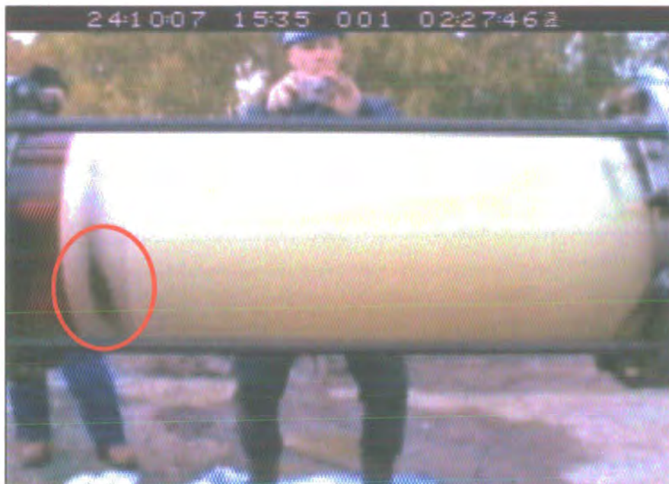
Figure 6.51. Initial contact between wax and pig in run 1.4a.
