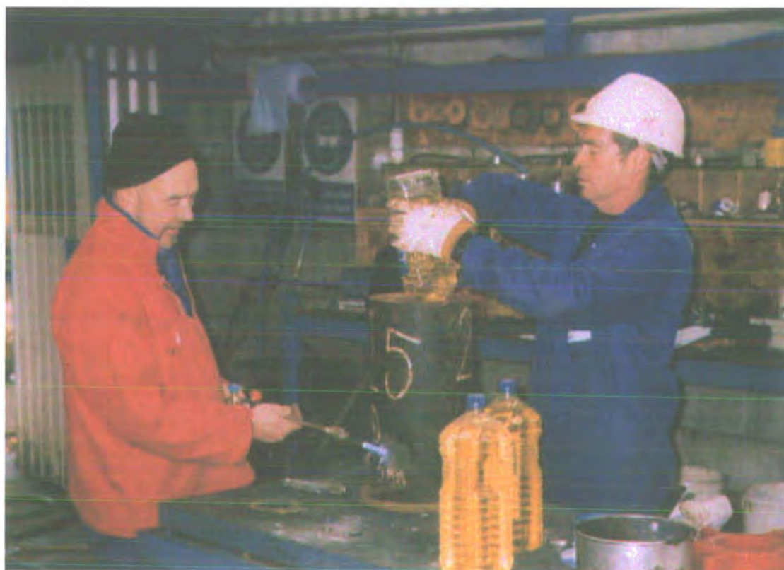
Figure 6.31. Mixing of oil and wax for sample preparation.
