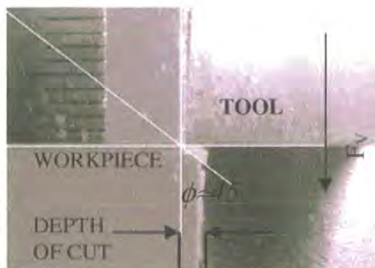
Figure 4.33.1. Observed shear angle ( \phi ) during the cutting of wax with a neutral rake tool, 1mm depth of cut.
