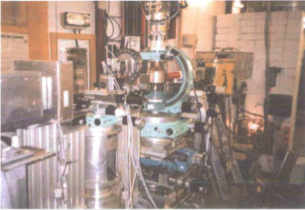
Figure 2.35: Picture of the BW5 Diffractometer when the Eulerian cradle is in use
