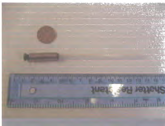
Figure 2.5: The pressure cell used for the SQUID measurements at raised pressure.
