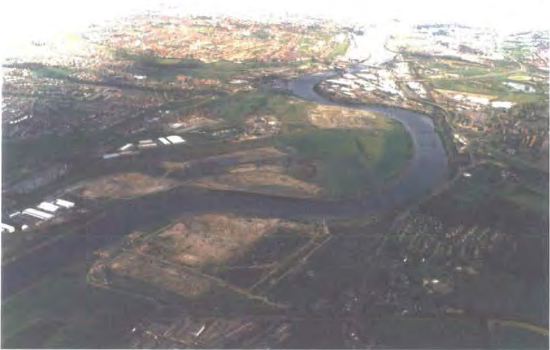
Fig. 31 Newburn Haugh – the loop in the river was dammed by the Tyne Commissioners to widen and deepen the river to make it passable by large boats. Dent's Meadow, the extensive island in the River Tyne immediately to the south of Newburn Haugh, which can be seen on the first edition Ordnance Survey map, fig. 238, was dredged away (copyright Air Images n.d.).
