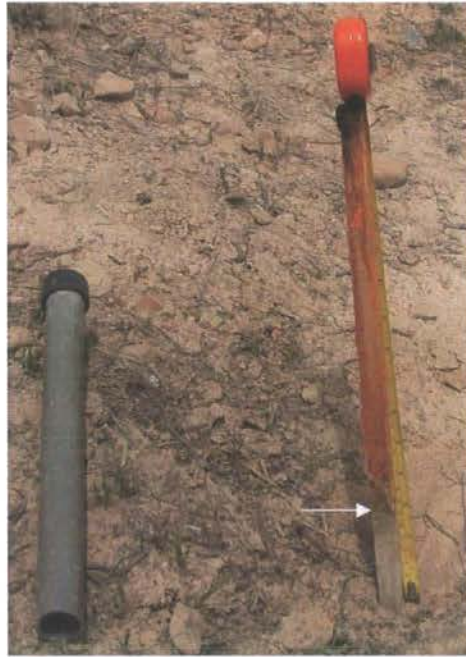
Figure 4.7. Flow depth measurement using the mini-crest stage gauge discussed here. Note that the cover has been removed for measurement.
