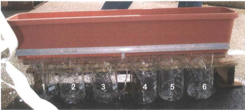
Figure 4.4. An experiment to assess the spread of discharge supplied to the top of the plot. Beakers numbered from left to right (1–6).
