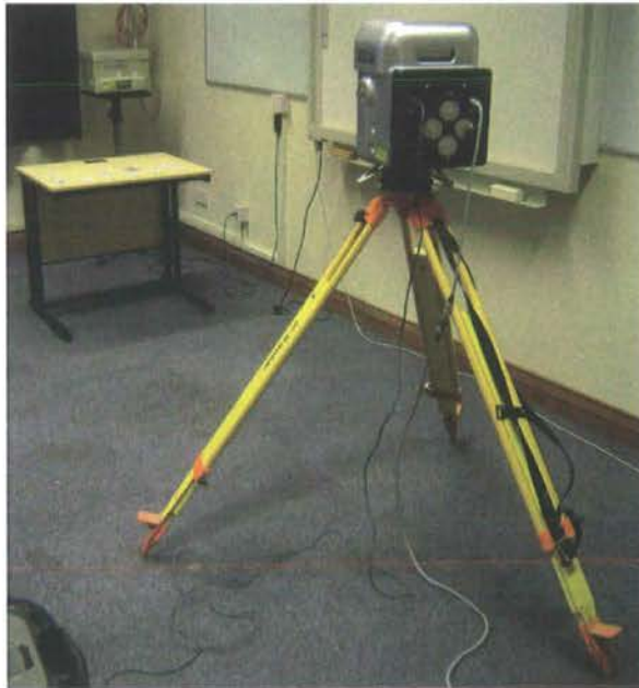
Figure 4.10. Experimental setup to establish the absolute precision of the GS200 laser scanner at the plot scale.
