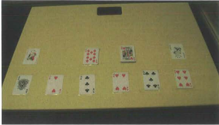
Figure 4.12. Card arrangement used to investigate scanner precision (from the viewpoint of the laser scanner). The card value represents the number in each stack on the front row. On the back row (from left to right) are card stacks of 1, 10, 20 and 1.
