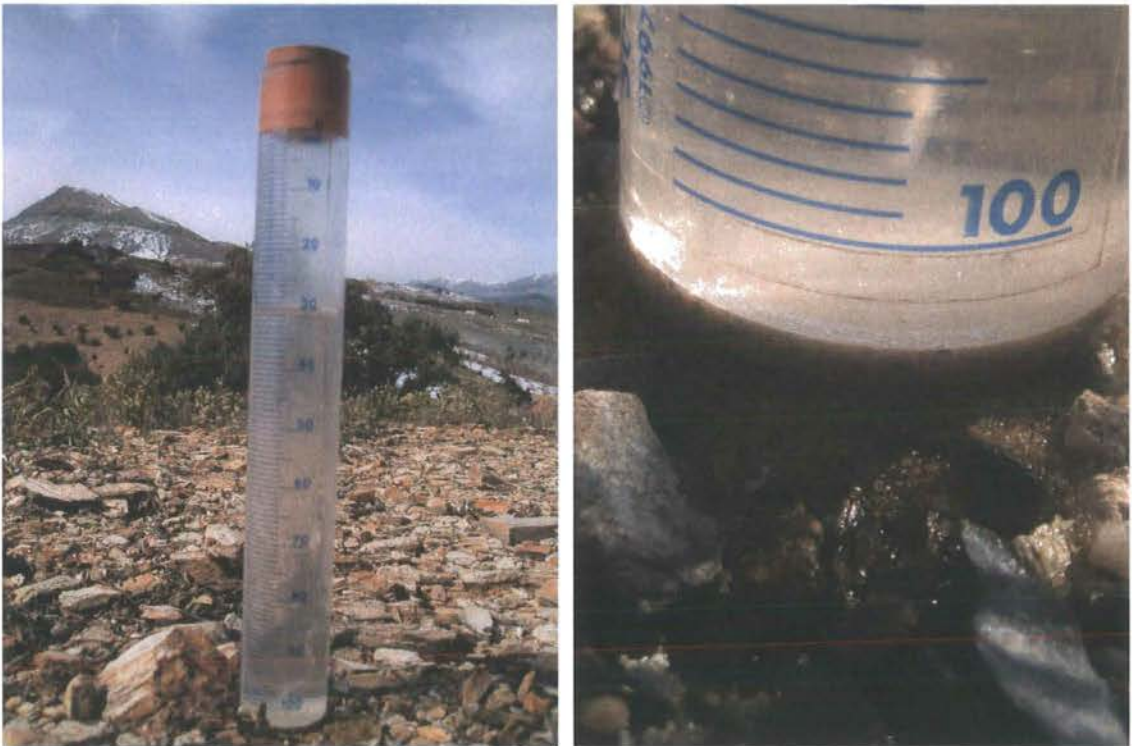
Figure 4.27. The minidisk infiltrometer (left) and the small layer of wet sand needed to ensure a good contact with the soil surface (right).
