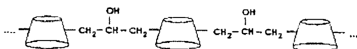
Figure 2.16: Structural sketch of poly- \beta -cyclodextrin derivative obtained by the cross linking of \beta -cyclodextrin monomers with 1-chloro-2,3-epoxy-propane
