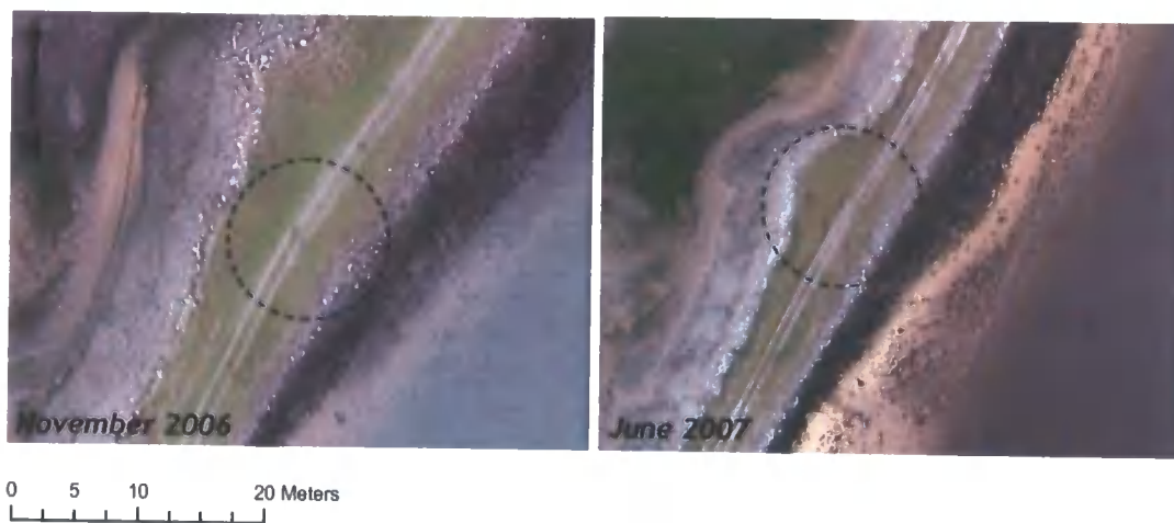
Figure 4.3 Inaccurate image 'stitches' produced by mosaicking process
