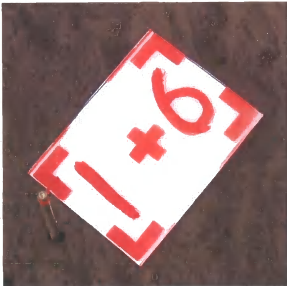
Figure 2.8 Panel used for ground control points (GCPs)
