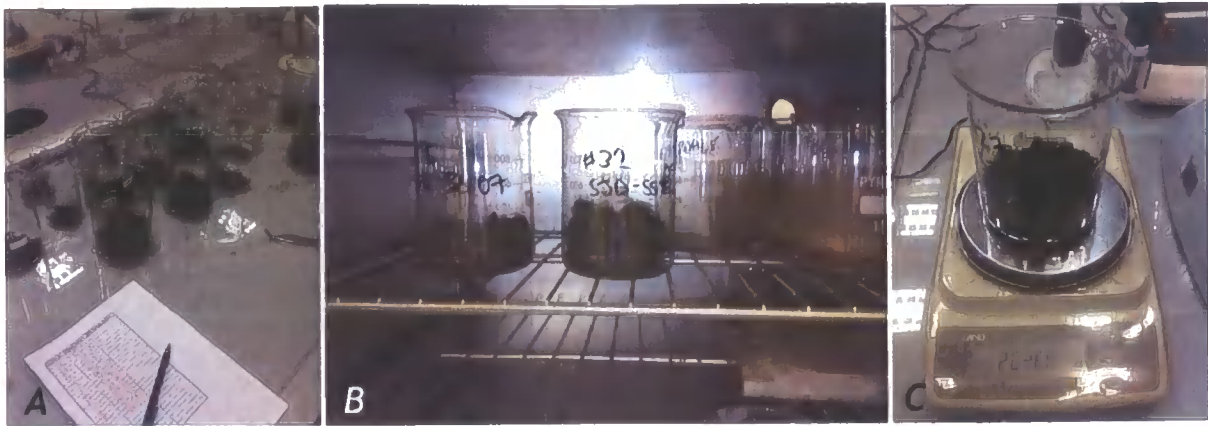
Figure 2.11 (A) Macroalgal samples were placed in beakers, (B) dried in oven and (C) weighed using analytical balance
