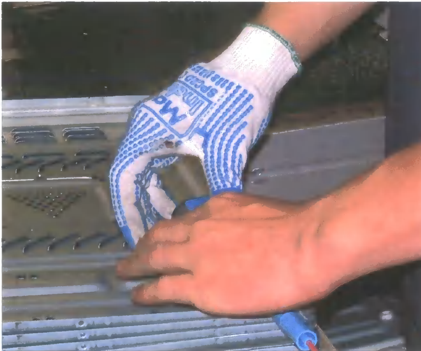
Illustration 5.4. The capacitor being clipped into place
