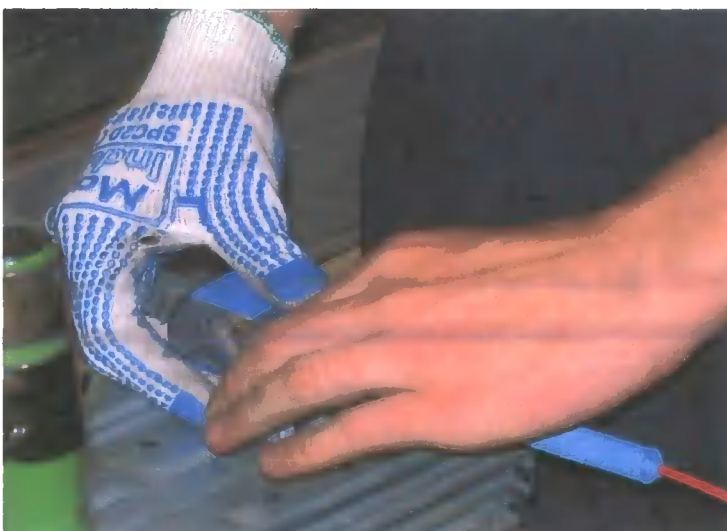
Illustration 5.5. Securing the capacitor
