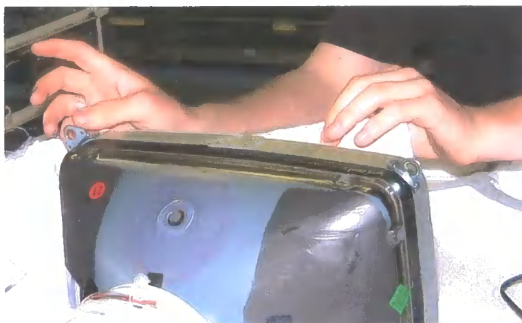
Illustration 5.8. Peeling the wrapper from the monitor front ready to lift the monitor – CDT prep
