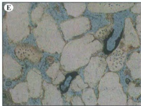
Grain dissolution porosity. WG-21, X10
