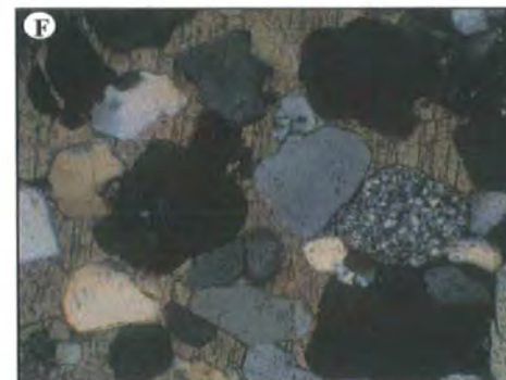
2mm Sedimentary rock fragment and mono quartz grains floating in carbonate cement. WG-38, X10
