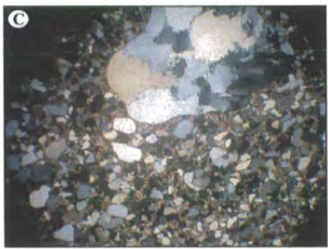
4mm Polycrystalline quartz grains, in carbonate cement. WG-17, X2
