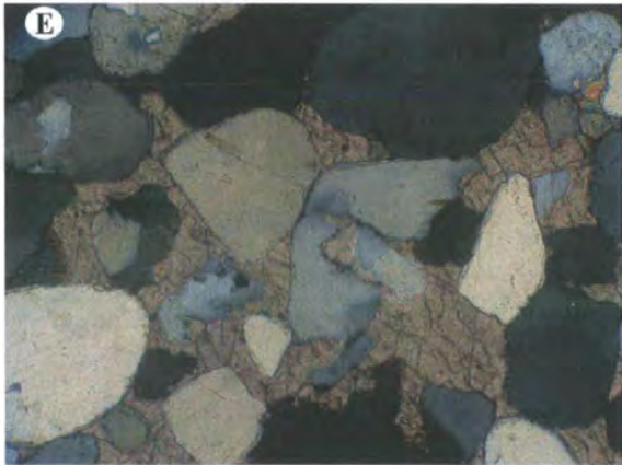
2mm Photo 3.3 Silica growth on the quartz grain surrounding by carbonate cemented. WG-38, X10
