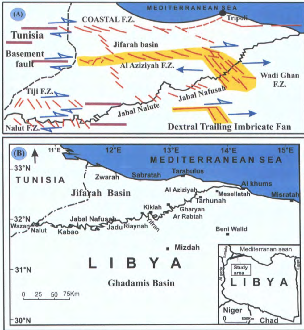
Fig. 1.7. Location maps of the studied area, Map (A); Interpretation of Al Aziziyah fault zone (Al Aziziyah F.Z.) and Wadi Ghan fault (Wadi Ghan F.Z.) in terms of dextral strike-slip faulting in studied area. Such a relation was used as a model to interpret the relationship between South Cyrenaica fault zone and Sirt basin rift (Source: Anketell and Ghellali, 1991; Anketell, 1996). Map (B) General location map of Jifarah Basin and surrounding area.
