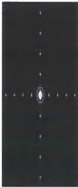
Figure 3.5 NAOMI theoretical diffraction-limited PSF showing diffraction pattern caused by DM segmentation. Intensity has been scaled to enhance diffracted orders.
