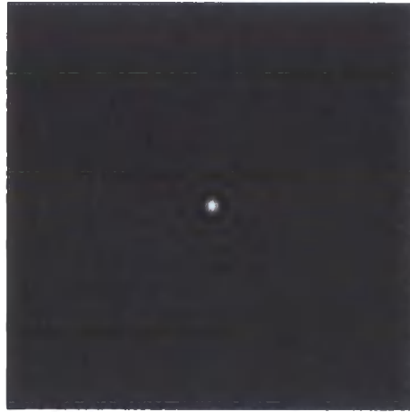
Figure 1.1 Diffraction limited Airy pattern formed at the focus of a telescope with circular aperture. The central obscuration present in most astronomical telescopes causes a slight increase in the diameter of the central core and a suppression of the intensity of the diffracted rings in comparison with the image presented above.
