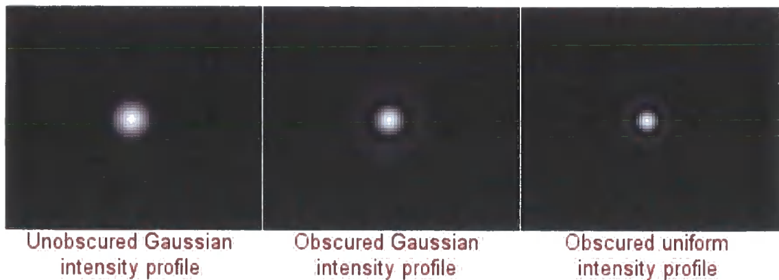
Figure 4.8 Focal points from obscured versus unobscured Gaussian input beams. Gaussian beams have been truncated at their 1/e^2 intensity points. Central obscuration diameter is 29% that of pupil diameter. The obscured pupil image formed by a uniformly illuminated intensity profile is included for comparison.
