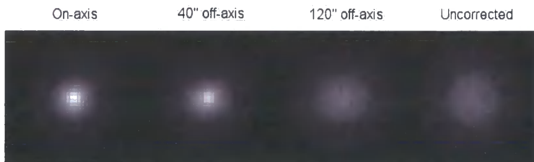
Figure 7.14 Sample PSFs taken from points in the field offset from the LGS and NGS by 0", 40" and 120" at a wavelength of 1250nm. Atmospheric r_0 is 0.14m. The uncorrected PSF is also shown. The square root of the intensity has been plotted to show fine structure in halo of the PSF. Intensities are to scale. Pixel scale is 0.031 arcseconds/pixel.
