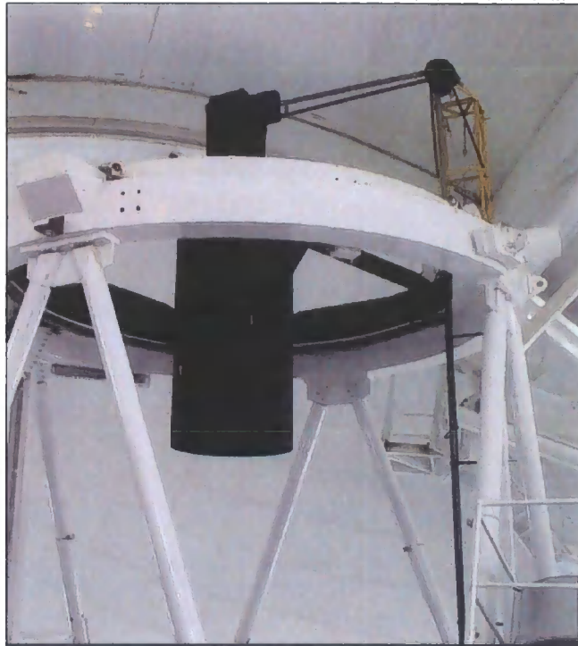
Figure 4.13 Enclosed beam path from WHT mirror cube to the BLT. Relay Mirror 2 is supported using the yellow-coloured structure attached to the top-end ring.
