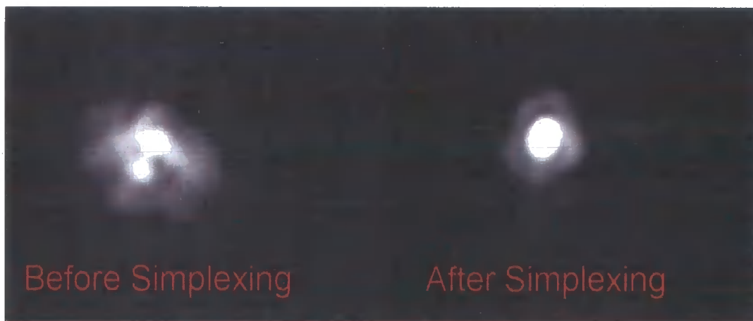
Figure 6.12 Effect of simplexing on the image quality at the science focus. First diffraction ring is visible in simplexed image.
