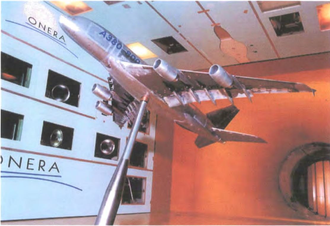
Figure 1.2.2, Airbus A380 under test at ONERA (2005).
