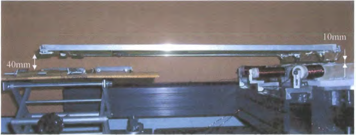
Figure 5.2.4 Hybrid Superconducting Magnetic Levitation System Levitating.
