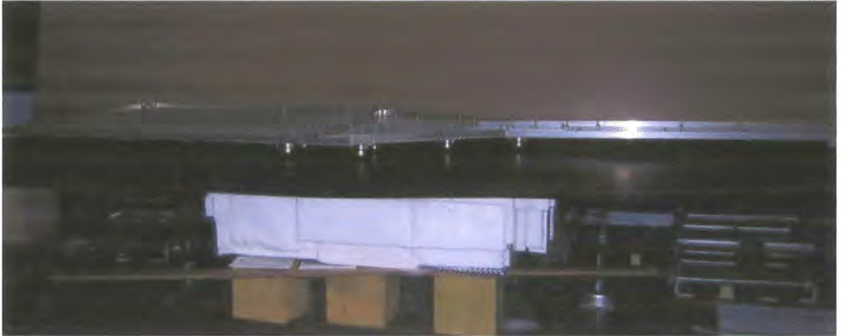
Figure 5.5.2, Superconducting Magnetic Levitation System with Aluminium Floor
