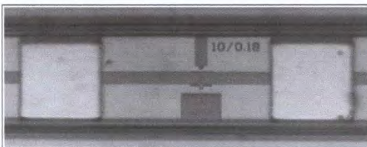
Figure 3.1: An image of 0.18\mu\text{m} n-channel device
