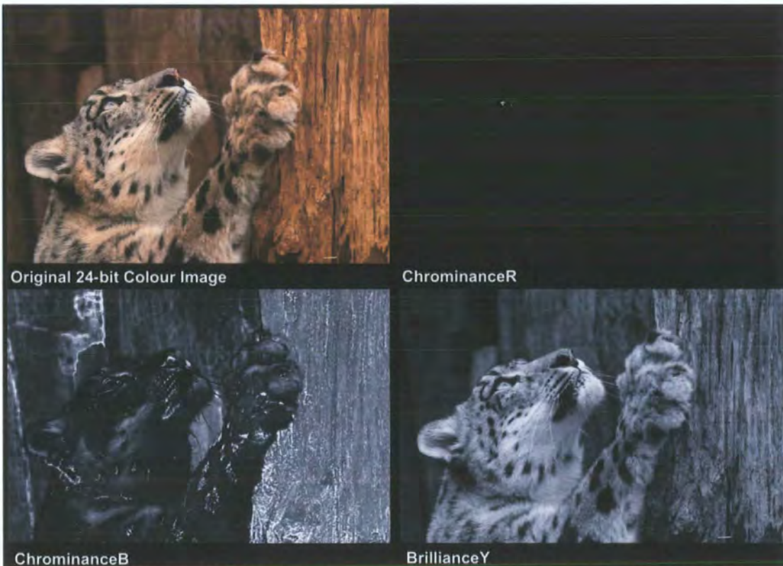
Figure 2.2.3.2: A colour bitmap separated into its YCbCr component channels
