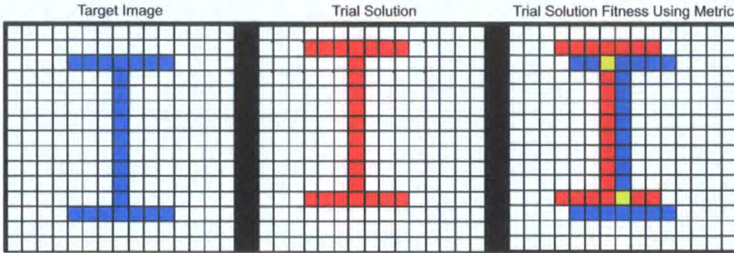
figure 2.4.5.1 – Weakness of simple image-comparison metrics for IFS searches
