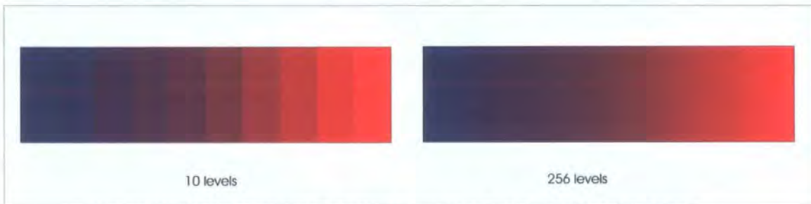
Figure 2.2.2: Greater colour depth allows more gradual tonal transitions
