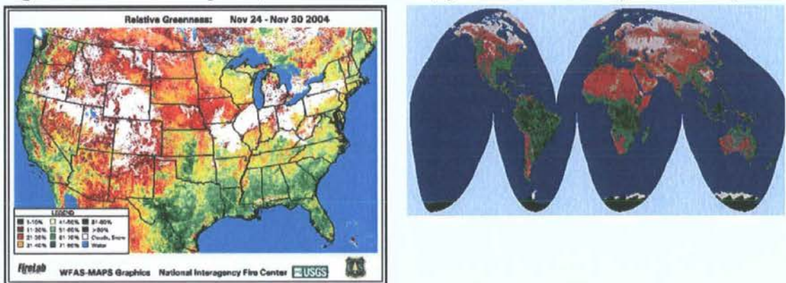
Figure 2.6 Thematic maps at a) continental 8 and b) global 9 scale: NDVI greenness maps
