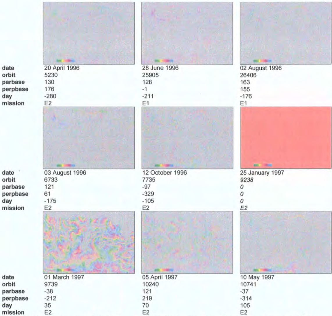
Figure 5.2: 35 interferograms of the Boulby area, colours showing the relative change in phase between neighbouring pixels.
