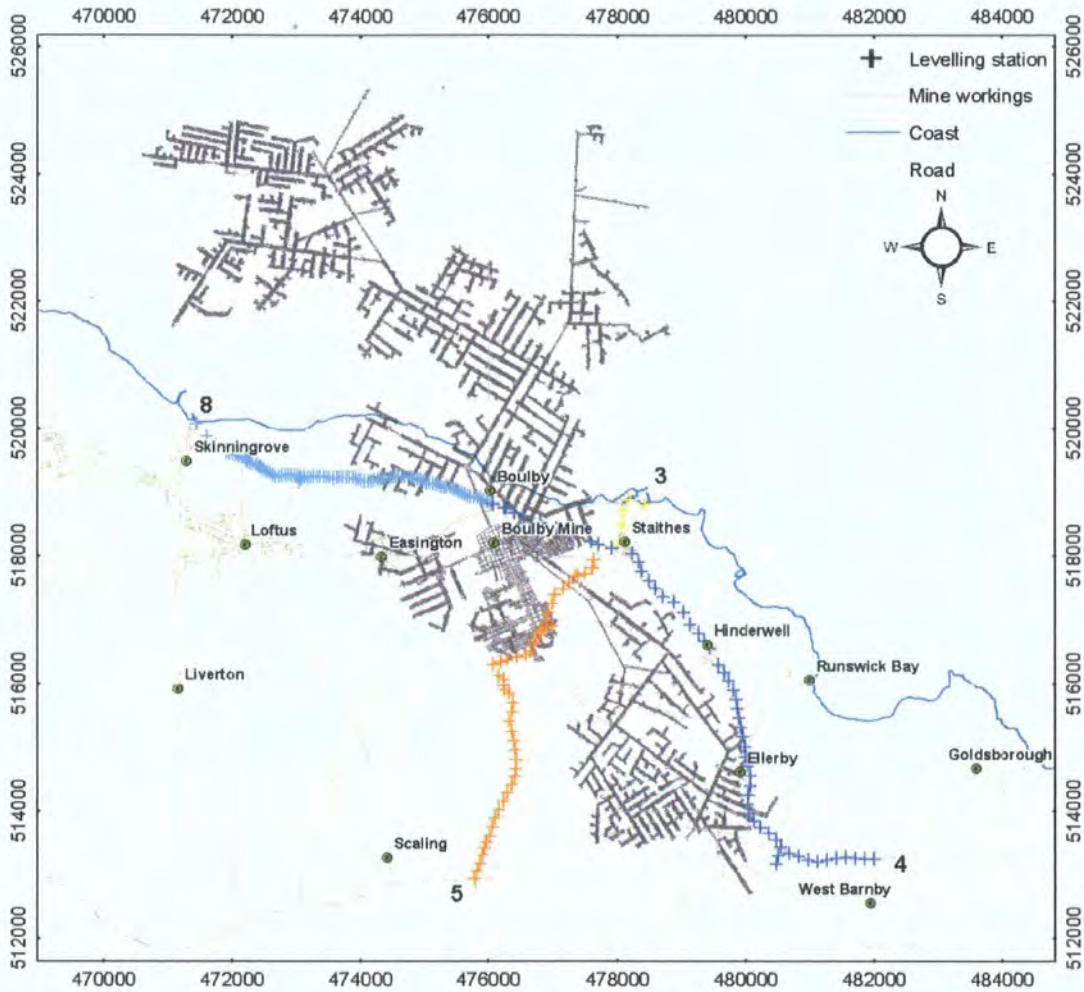
Figure 5.27: Levelling stations on lines 3, 4, 5 and 8 crossing the Boulby area
