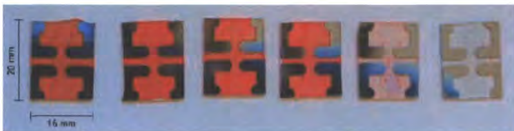
Figure 2.4 The devices (left to right) 100%, 80%, 50%, 30%, 5% MEH-PPV and pure 202
