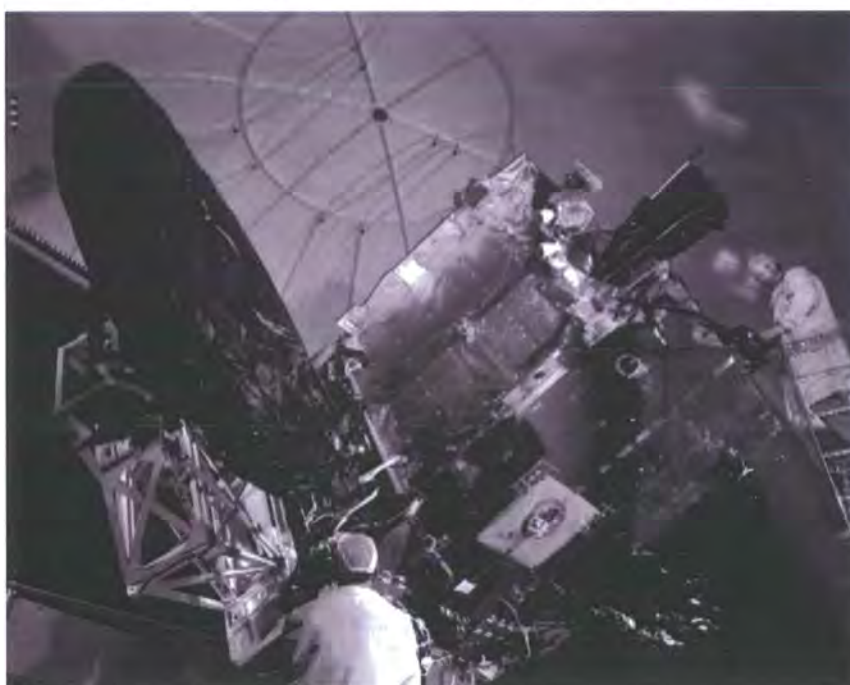
Figure 3.10 HotBird Satellite Undergoing Final Testing.
