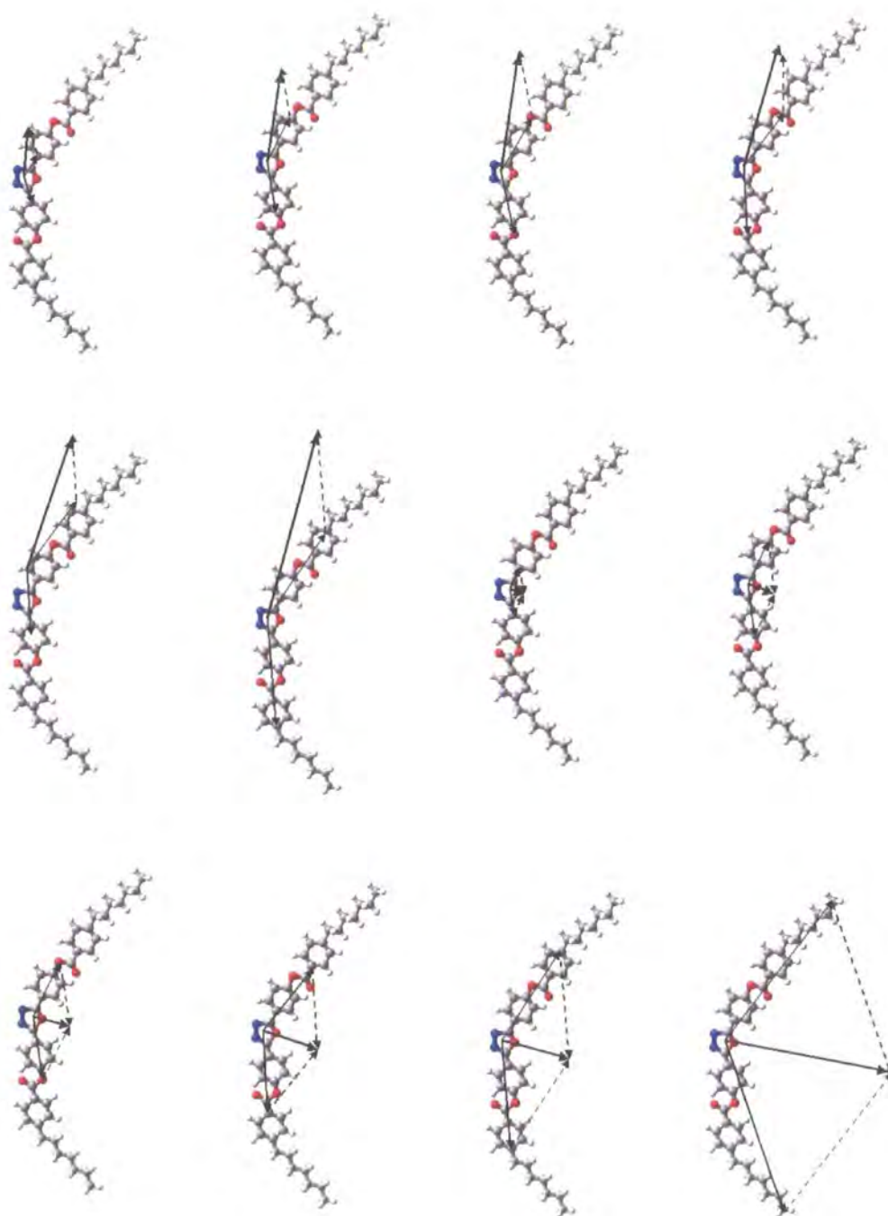
Figure 3.17: Some of the vectors used to define the orientation of the molecule ODBP-Ph-C 7 .
