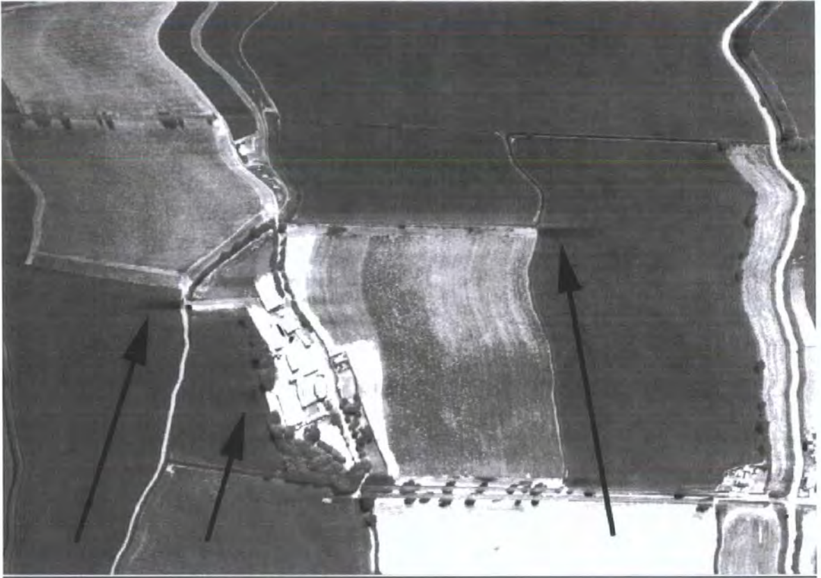
Figure 47 Thermal “shadows” caused by destripping the day time thermal raw ATM data
