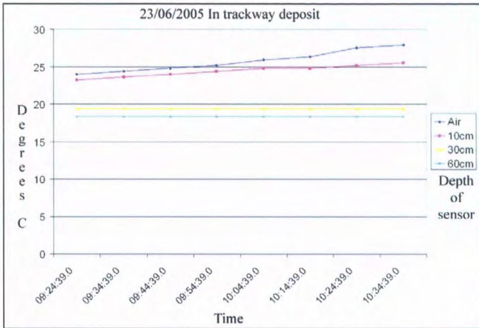
Figure 90 Temperature results from the logger buried within the open sand deposit (day)
