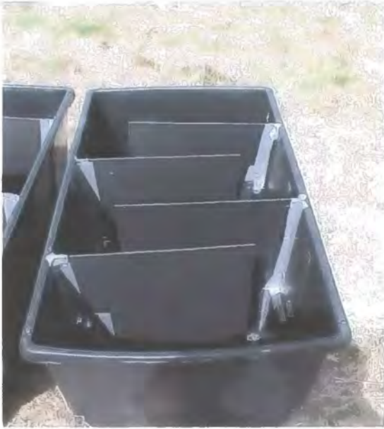
Plate 2.1. A test tank prior to addition of gravel and reeds
